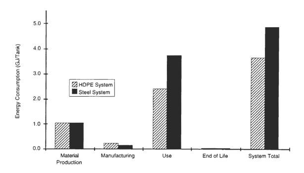
Figure 4-1. Life Cycle Energy Consumption for HDPE and Steel Tank Systems
