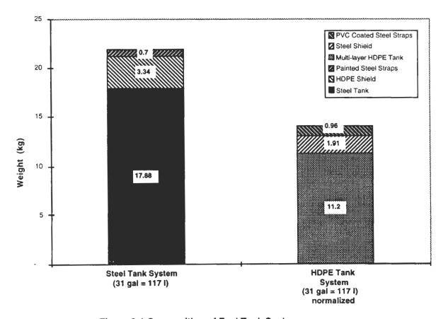
Figure 2-1 Composition of Fuel Tank Systems
