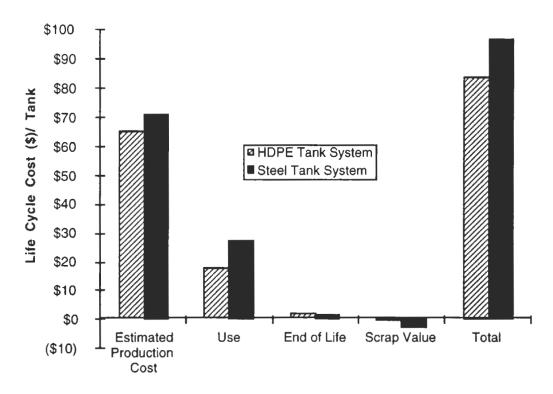
Figure 4-12. Life Cycle Costs of Fuel Tank Systems
