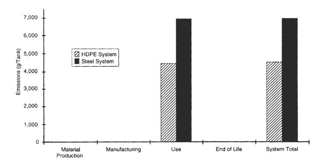
Figure 4-4. Life Cycle Carbon Monoxide Emissions for HDPE and Steel Tank Systems
