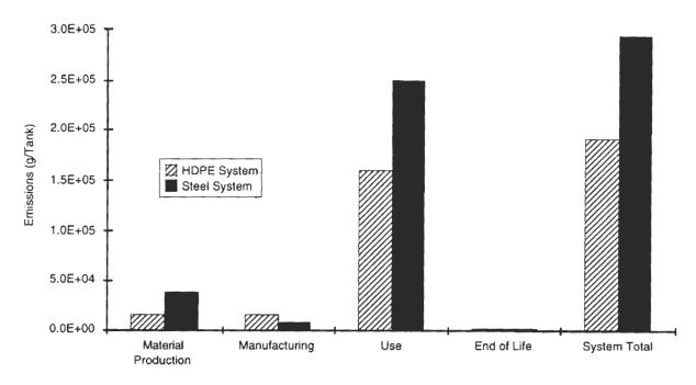
Figure 4-3. Life Cycle Carbon Dioxide Emissions for HDPE and Steel Tank Systems
