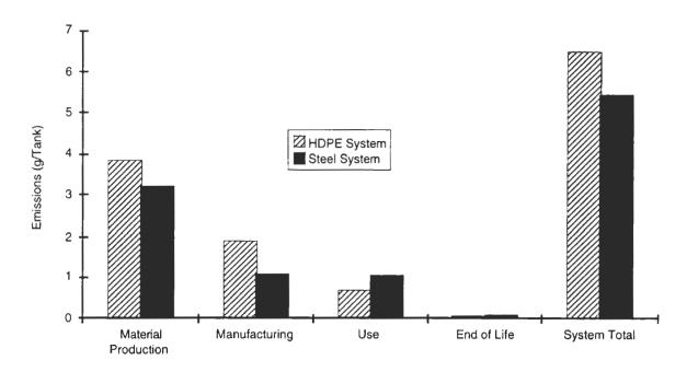
Figure 4-11. Life Cycle Waterborne Metals Emissions for HDPE and Steel
