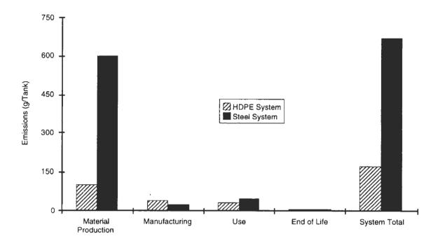
Figure 4-6. Life Cycle PM Emissions for HDPE and Steel Tank Systems
