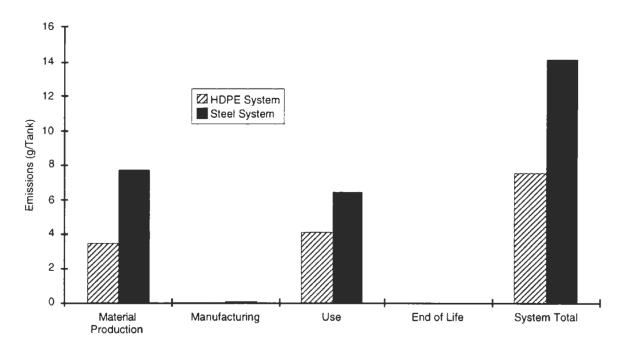
Figure 4-9. Life Cycle Suspended Solids Emissions for HDPE and Steel Tank Systems
