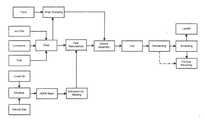
Figure 2-2. Steel Fuel Tank System
