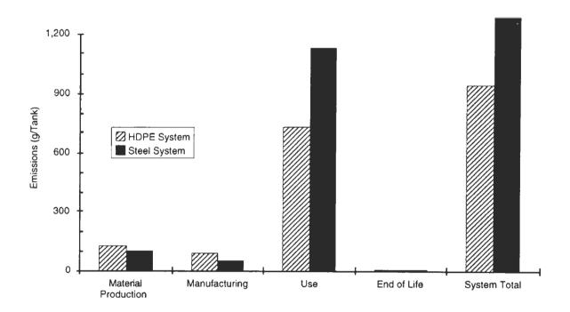
Figure 4-5. Life Cycle NOx Emissions for HDPE and Steel Tank Systems
