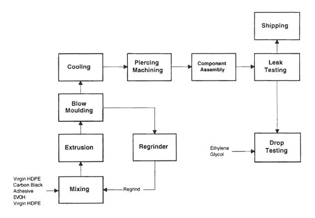
Figure 3-2 Multilayer Plastic Fuel Tank Manufacture
