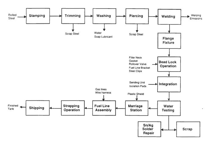
Figure 3-1 Steel Tank Manufacture
