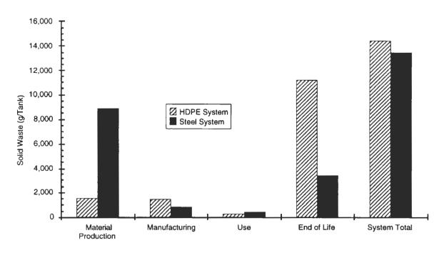
Figure 4-2. Life Cycle Solid Waste Generation for HDPE and Steel Tank Systems
