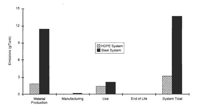
Figure 4-10. Life Cycle Waterborne Oil & Grease Emissions for HDPE and Steel Tank Systems
