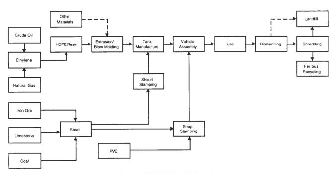
Figure 2-3. HDPE Fuel Tank System
