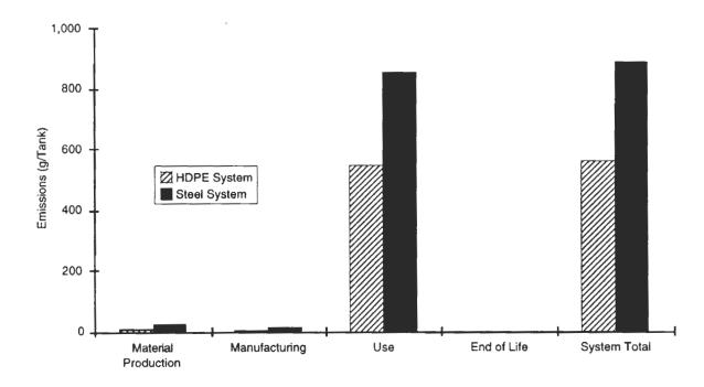
Figure 4-8. Life Cycle Dissolved Solids Emissions for HDPE and Steel Tank Systems
