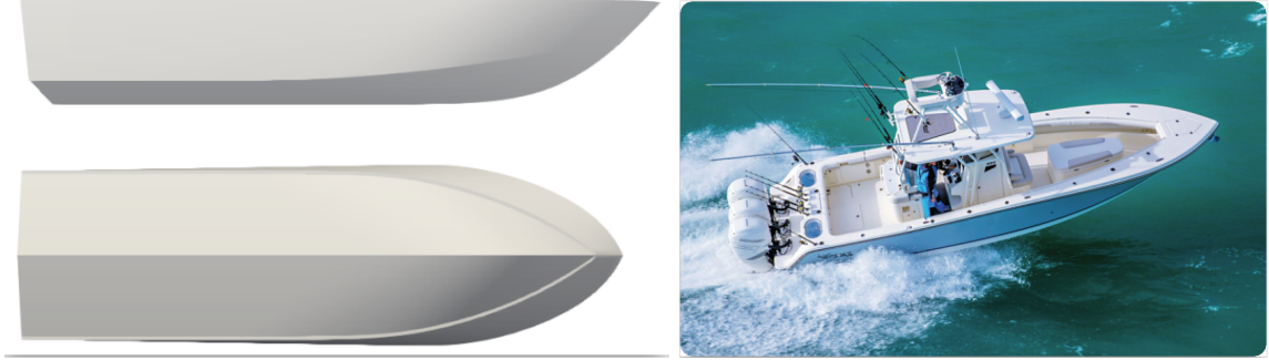
Figure 2.4: Left is a schematic of the GPPH model. Right is a photo of a planing boat.
