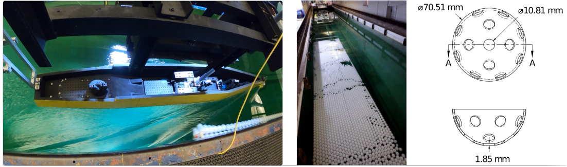
Figure A.2: From left to right are (left) Snapshot of the ship model traveling at a constant speed of Fr = 0.29 , (middle) image of the raft consisting of Whiffle balls, (right) drawing of the perforated spherical shell.
