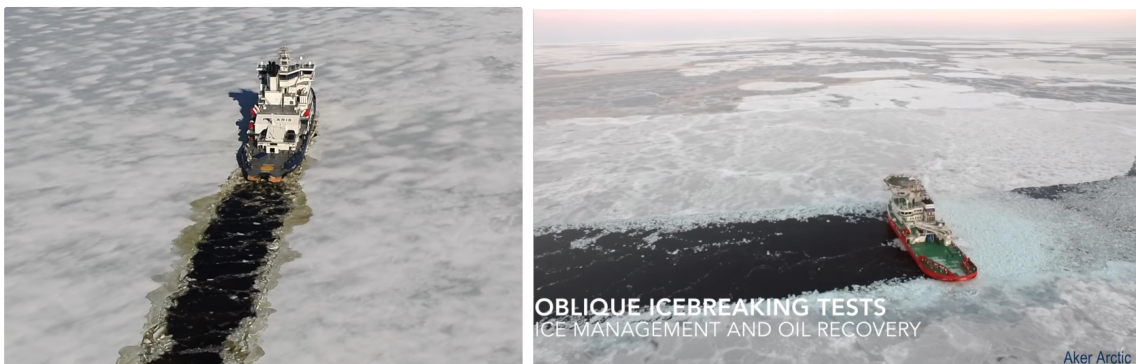
Figure 1.7: Ice-breakers creating open-water ice channels either in straight-ahead or oblique mode. Pictures courtesy of Aker Arctic.
