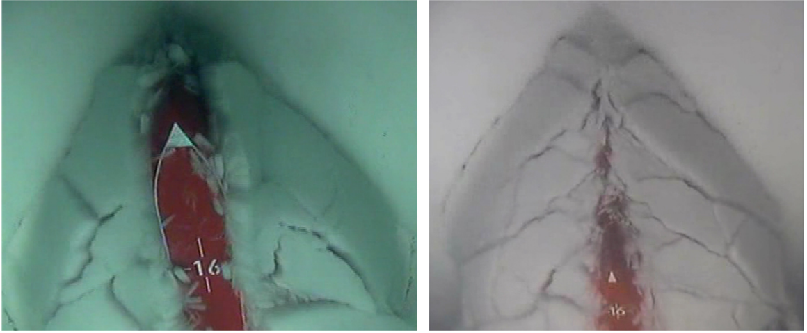
Figure 1.4: Breaking patterns of model ice under water with two different ship models. From Fig. A6. in Myland and Ehlers (2016) .
