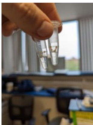
Figure 4.14 Minimized Counter Diffusion Assembly. Set up as shown in Figure 4.13 with 20 mm and 0.3 mm OD capillaries.
