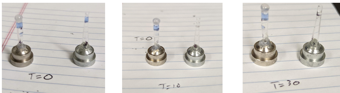
Figure 4.10 Feasibility of Custom Capillary Mounts. A time trial of sealed capillary containing methyl viologen oxygen indicator with a snapped capillary exposed to oxygen as a control. Once the capillaries were brought out of the anaerobic chamber, we snapped our control at T=0 min. After 10 min our control turned colorless, but the methyl viologen solution stayed violet in the sealed capillary over 3 days.
