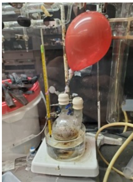
Figure A2 Copper sulfate mediated synthesis with 1,2-ethanedithiol. Inert gas balloon was used to attach the round bottom to avoid oxidative damage to the catalyst while all compounds were degassed on a Schlenck line.
