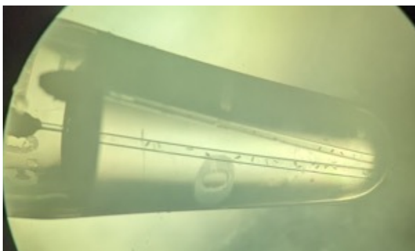
Figure 4.14 Minimized Counter Diffusion Assembly. Set up as shown in Figure 4.13 with 20 mm and 0.3 mm OD capillaries.
