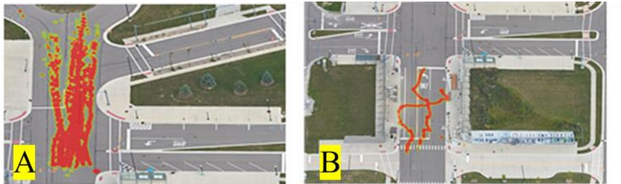
Figure 7.2 (A) GPS heatmap of six subjects jogging through MCity street - using GPS estimates from mapping module. (B) GPS heatmap of two subjects patrolling MCity street and crossing paths – using GPS estimates from mapping module.
