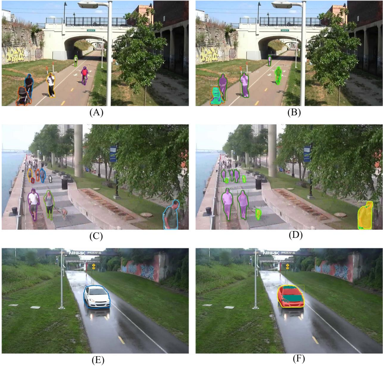
Figure 2.6 Performance of Mask R-CNN detector with manually annotated ground truth images (A, C, E) with different weather conditions (sunny, cloudy, rainy) and detector results (B, D, F).
