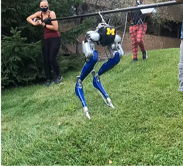
Figure 3.1: Cassie Blue using an ALIP-inspired MPC gait controller to walk sideways up a 22^\circ incline on wet grass. Lateral walking with Cassie is much more difficult than longitudinal walking due to tight workspace constraints, which are accounted for in our formulation.
