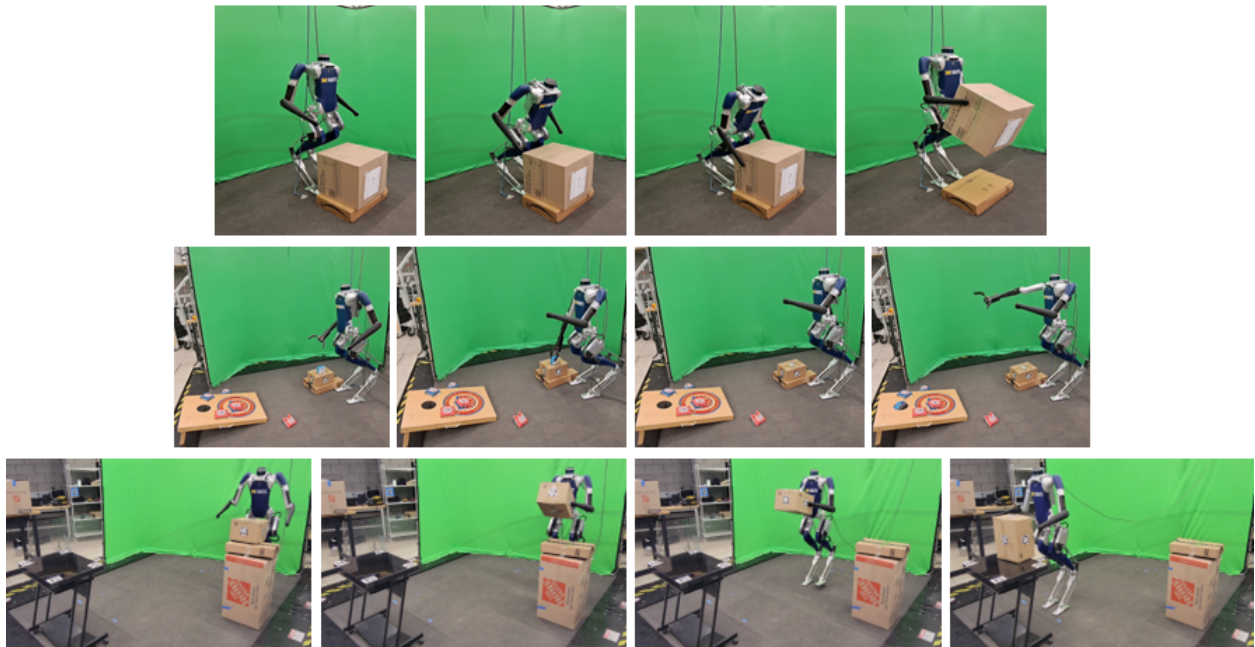
Figure 5.1: A Digit robot executes a variety of whole-body motions using the Kinodynamic Fabrics Framework. (Top) Digit lifts a bulky box of non-uniform, shifting mass distribution that the framework does not model. (Middle) Digit plays cornhole. (Bottom) Digit transports a package to a desired location. Digit is designed by Agility Robotics.
