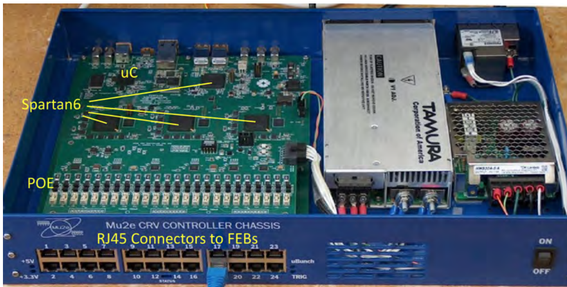
Figure 4.13: Photograph of a CRV ROC. The main components are labeled in yellow [17]. The 24 RJ45 Ethernet connectors on the bottom of the board connect to the FEBs. The final ROC design is essentially identical to the initial design.
