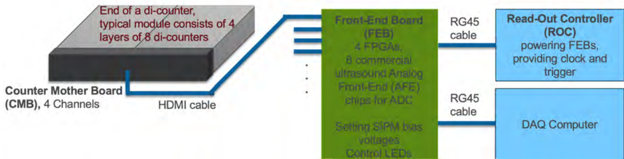
Figure 6.2: Wideband test bench electronics diagram. A block diagram of the electronics used to record data at the Wideband test bench [5]. Each block is labeled, beginning with a CMB on the left, an FEB in the center, and a ROC on the right. Short descriptions accompany each block.
