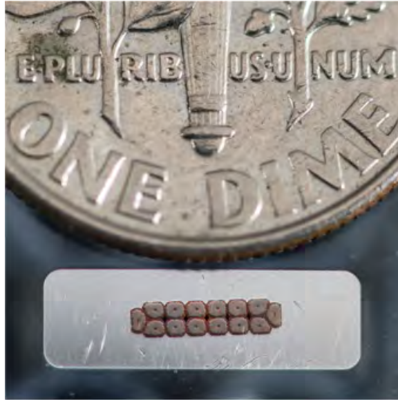
Figure 3.5: Superconducting solenoid cable cross-section. A cross-section look at the superconducting, aluminum-stabilized Nb-Ti cable used to wind the Mu2e solenoids [7].
