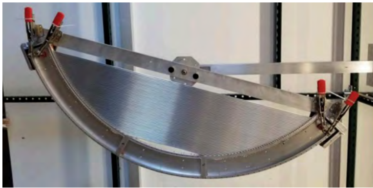
Figure 3.10: Photograph of a Mu2e tracker panel. Each panel contains 2 layers of 48 straws, staggered to reduce gaps. The outer ring of the panel in this photograph does not contain any electronics [15].
