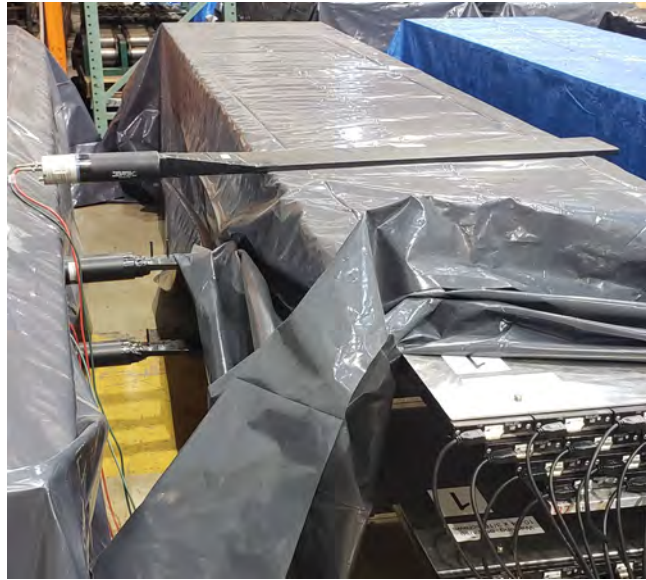
Figure 6.3: Photograph of the Wideband test bench trigger paddles. A photograph of the CRV module stack containing module 127 and the trigger paddles surrounding module 127. The three PMTs at the ends of the three trigger paddles are visible on the left side of the image. The top trigger paddle is visible as the black wrapped bar laying across the top of the stack. The lower 2 paddles also lay across the stack, aligned underneath the top trigger paddle for maximum overlap.
