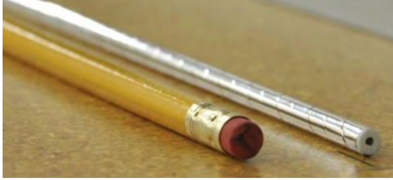
Figure 3.9: Straw tube details. A photograph of a Mu2e tracker straw next to a standard sized pencil. Each straw in the tracker is thinner than a pencil. Aluminum coating in a wound pattern is visible on the outside of the straw [14].
