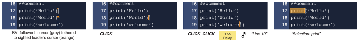
Figure 4.2: Image shows BVI developer’s code editor as she follows a sighted leader. CodeWalk tethers the cursors of collaborators in Follow mode. When the sighted leader uses arrow keys to navigate, CodeWalk plays skeuomorphic keyboard sounds for each line moved. When they stop navigation at line 19, CodeWalk plays an artificial falling tone to indicate downward movement followed by line number announcement. Similarly, when they highlight a word, CodeWalk announces the selection.
