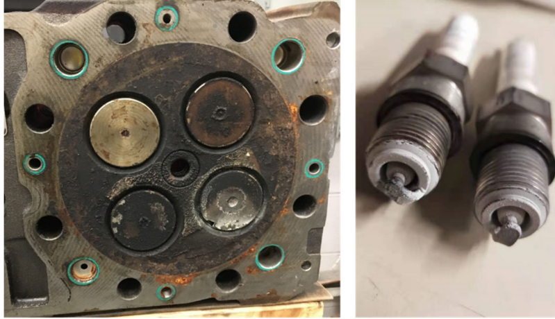
Figure 2.3 Photos of landfill gas piston engine parts showing white powder deposits attributed to silica. Left: cylinder head after scrubbing and cleaning to remove deposits. Note the damage to the valves due to particle accumulation; Right: spark plugs showing white particle accumulation attributed to silica.
