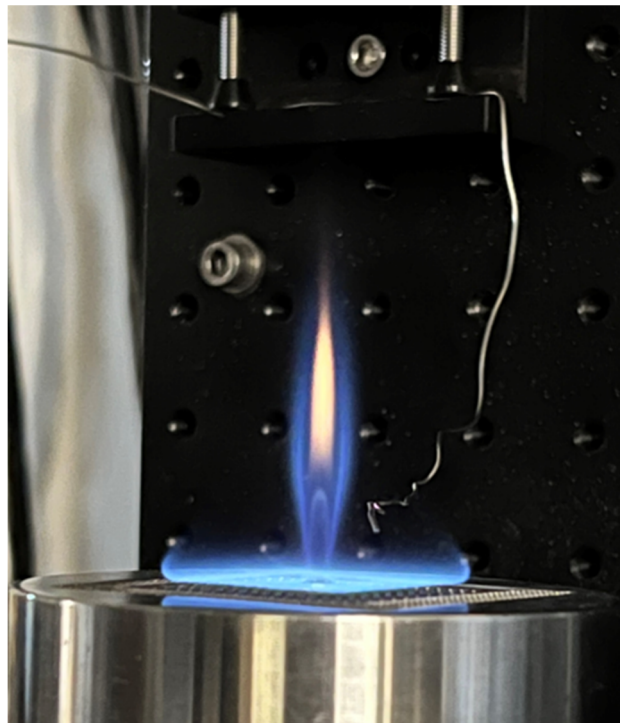
Figure 4.4 Photo of methane flat flame ( \Phi = 1.0 ) with HMDSO flame at the center of the burner.
