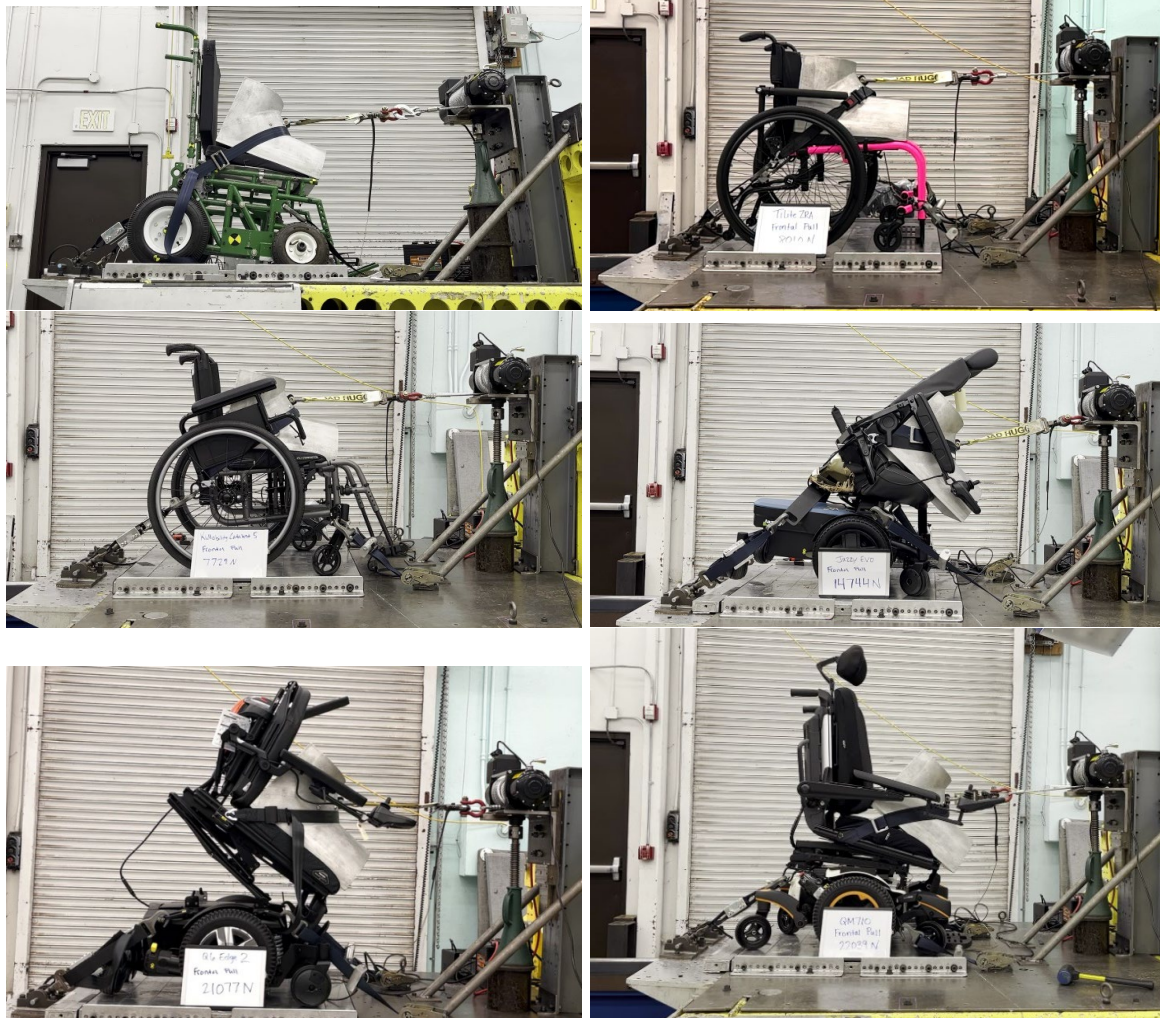
Figure 39. Photos of peak frontal static loading for SWCB (upper left), TLZ (upper right), KMC5 (middle left), JCS (middle right), QE2 (lower left), and SQ710 (lower right.)
