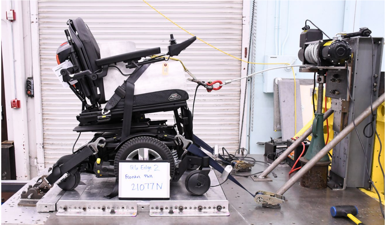
Figure 26. Example setup for frontal static pull test of QE2.
