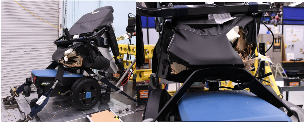
Figure 42. Damage to JCS sustained during lateral static testing.
