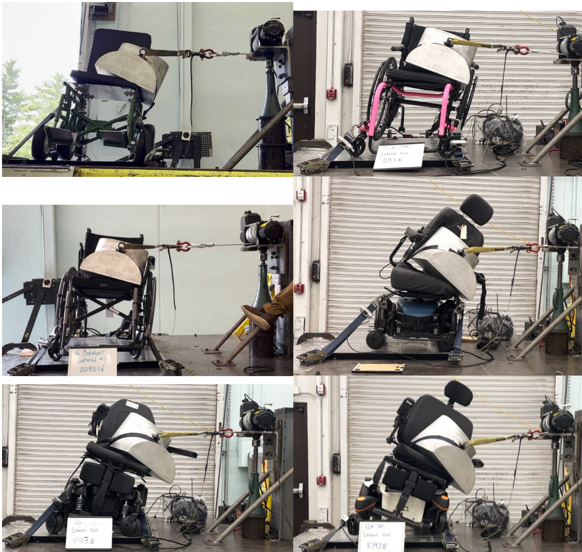
Figure 35. Photos of peak lateral static loading for SWCB (upper left), TLZ (upper right), KMC5 (middle left), JCS (middle right), QE2 (lower left), and SQ710 (lower right.)
