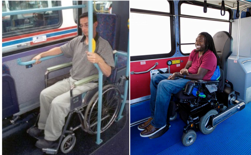
Figure 3. Rear-facing wheelchair passenger station (left) and Q'Straint Quantum automated docking system (right).
