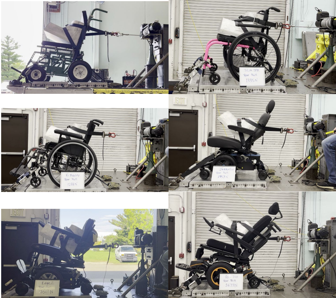
Figure 31. Photos of peak rear static loading for SWCB (upper left), TLZ (upper right), KMC5 (middle left), JCS (middle right), QE2 (lower left), and SQ710 (lower right.)
