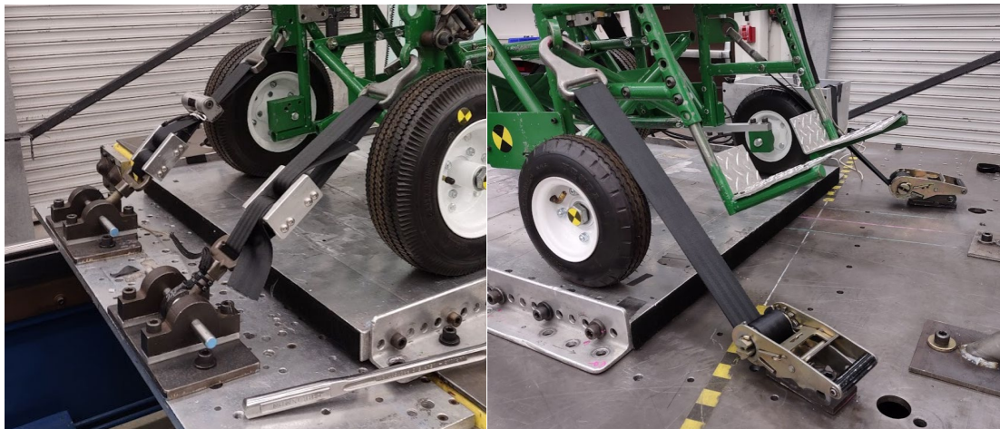
Figure 14. Rear (left) and front (right) SWTORS used to secure wheelchairs during WC19 testing.
