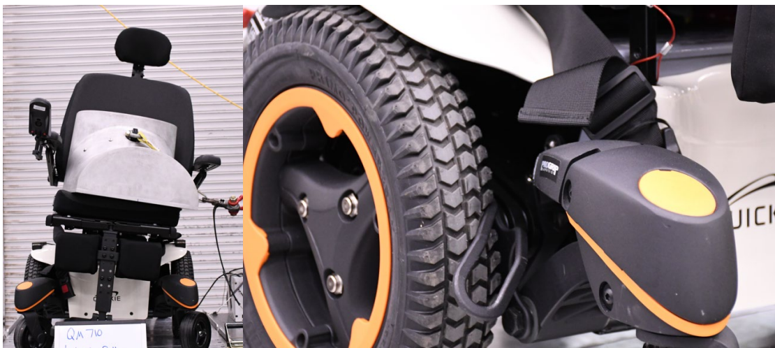
Figure 38. Damage to SQ710 sustained during lateral static testing.
