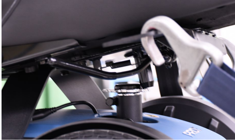
Figure 34. Closeup photo of JCS seat detached from base after upward loading test.
