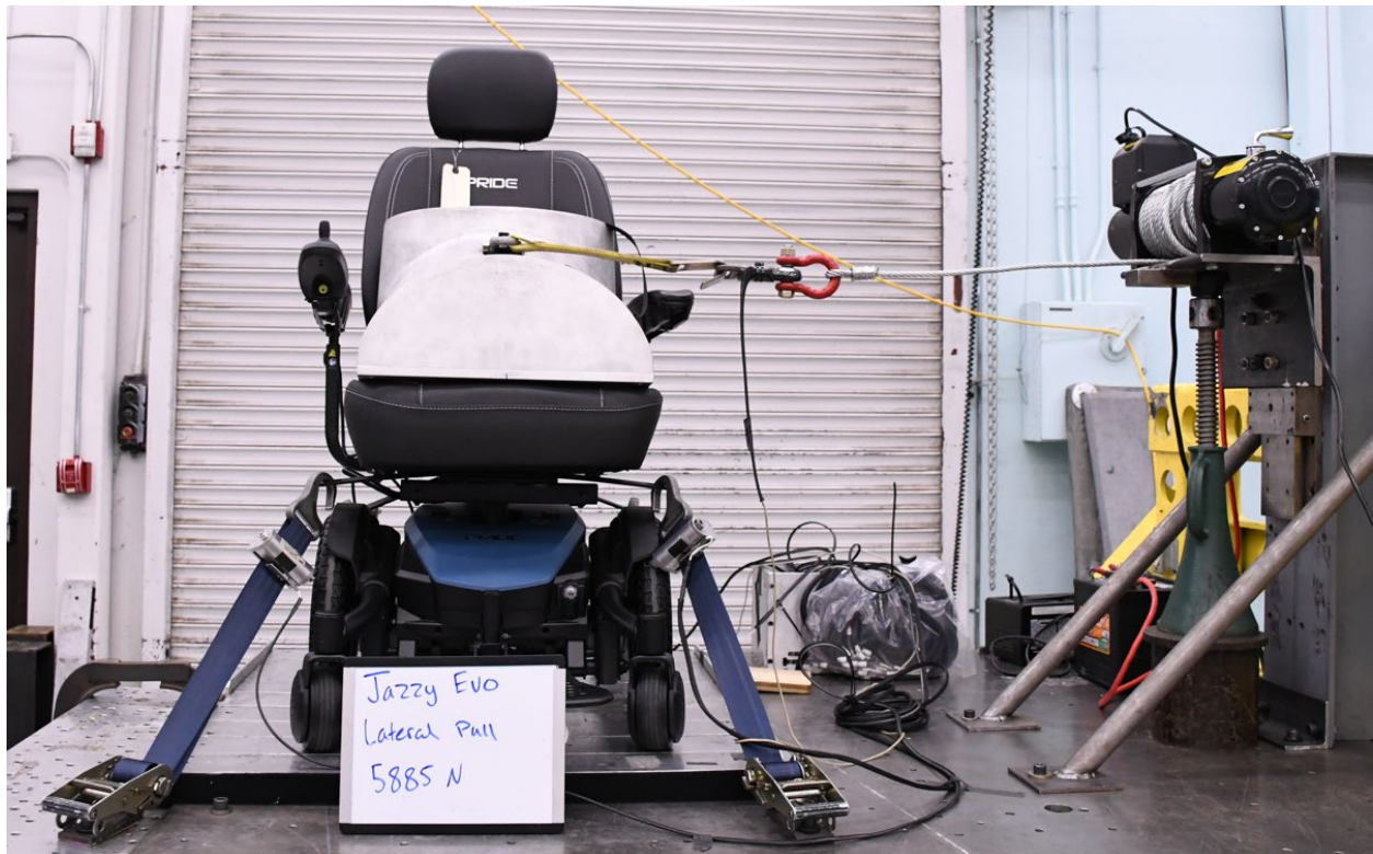
Figure 28. Example setup for lateral static pull test of JCS.
