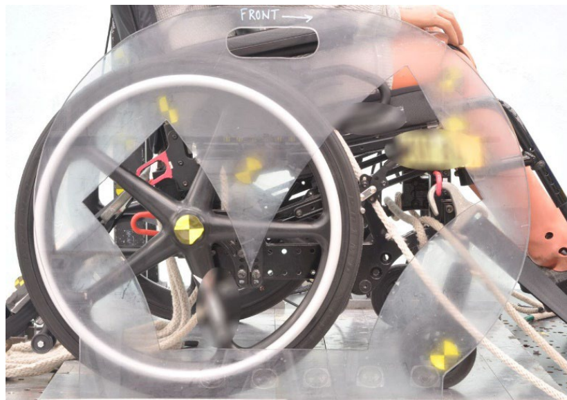
Figure 8. Fixture used to check that wheelchair securement points are in recommended zone.
