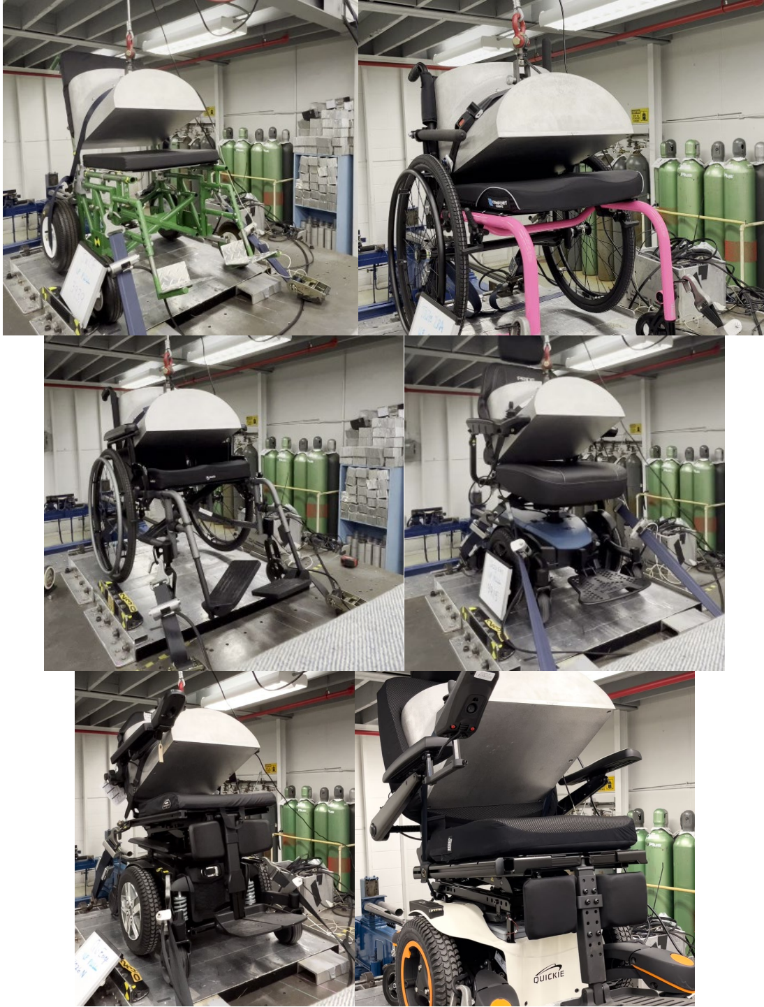
Figure 33. Photos of peak upward static loading for SWCB (upper left), TLZ (upper right), KMC5 (middle left), JCS (middle right), QE2 (lower left), and SQ710 (lower right.)
