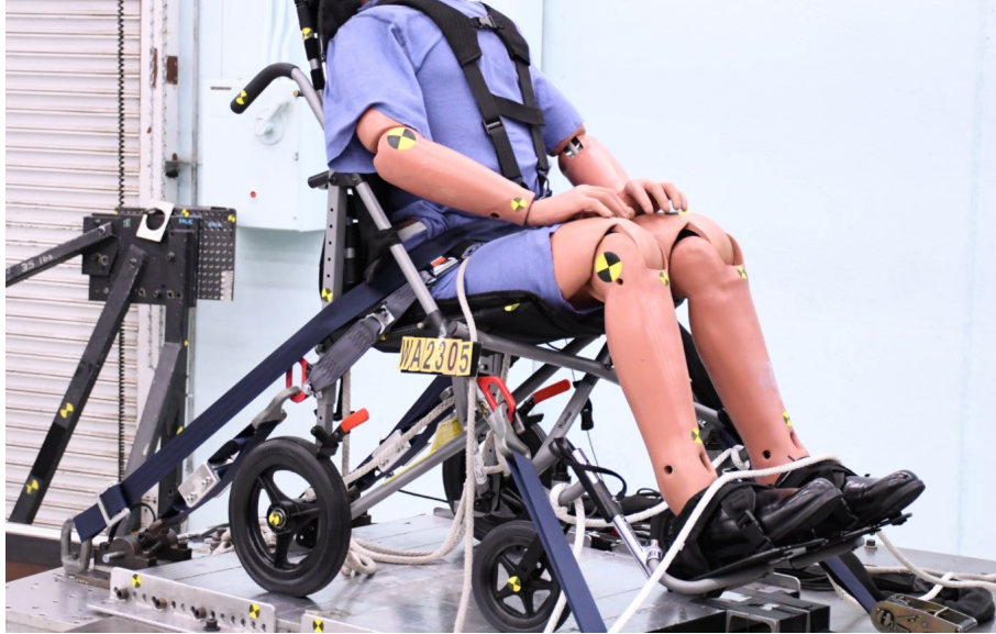
Figure 48. Example of ATD secured by both wheelchair-anchored lap belt and vehicle-anchored lap belt.
