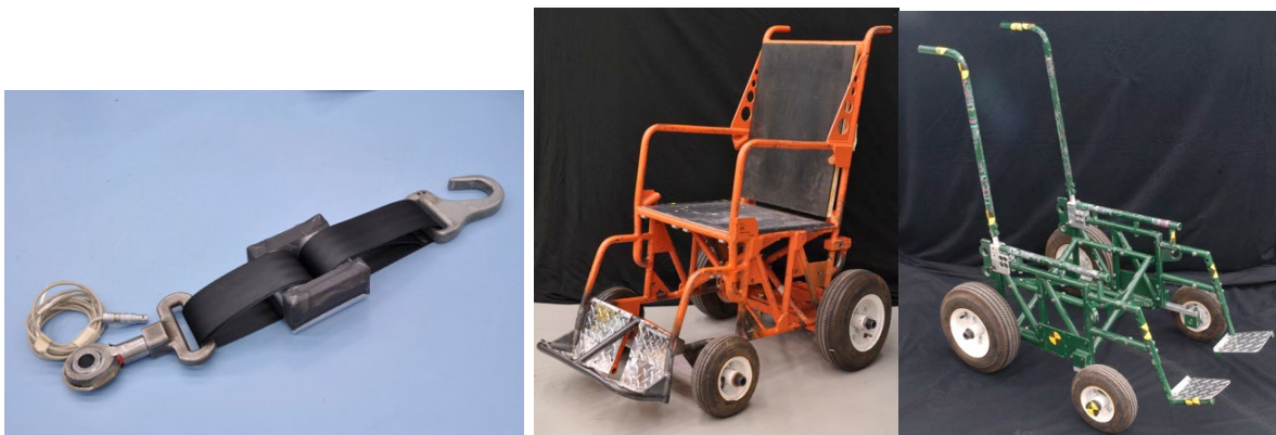
Figure 6. Surrogate wheelchair tiedown (left), surrogate wheelchair (center), and surrogate wheelchair base (right).
