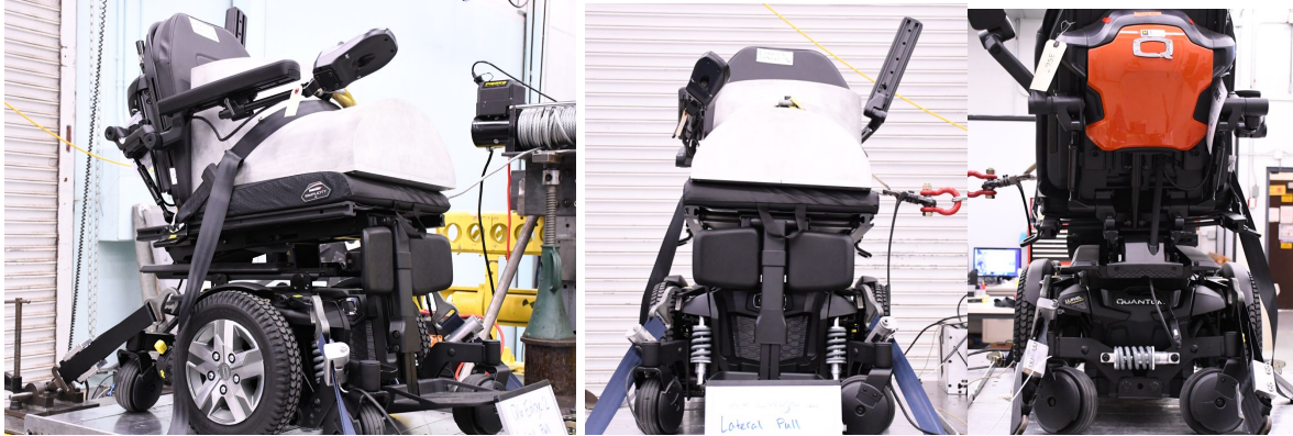
Figure 36. Damage to QE2 sustained during lateral static testing.
