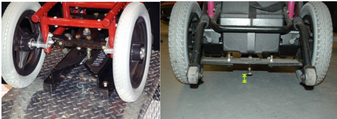
Figure 1. Examples of wheelchair engaged with docking system mounted to vehicle floor (left) and example of mating hardware with low ground clearance (right).
