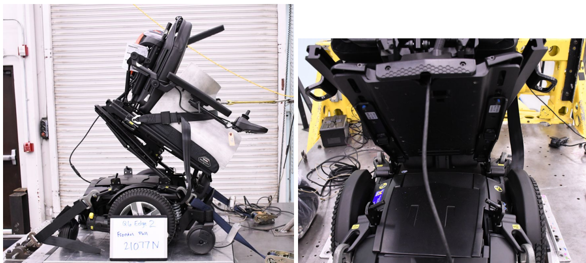
Figure 40. Damage to QE2 sustained during lateral static testing.
