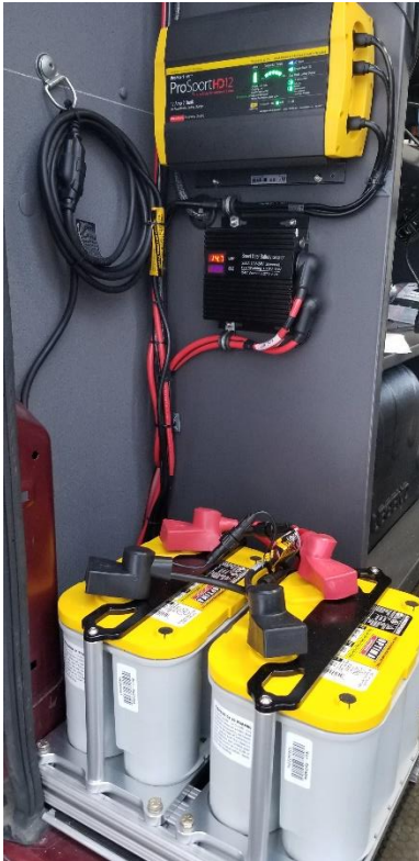
Fig 3. On-board Auxiliary batteries to power the active seat (with vibrotactile motors), computers, and instrumentation
