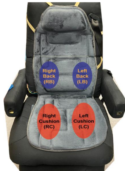
Fig 6. Active Seat with embedded Vibrotactile Motors
