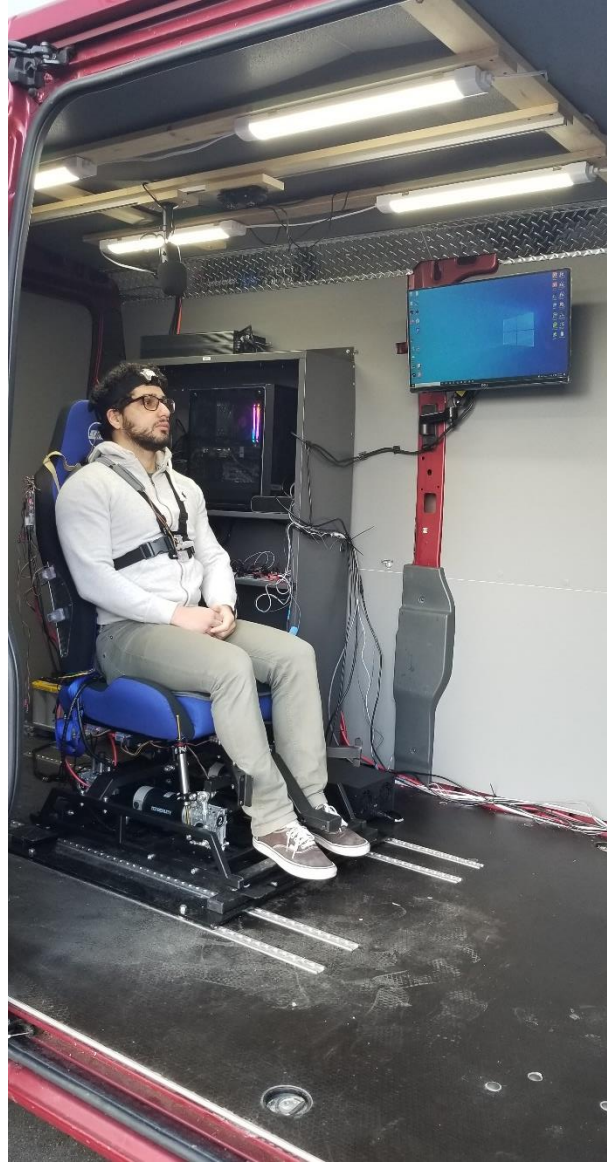
Fig 2. Vehicle Testbed: Cargo Space modified to include Active Seat, Display Panels, Instrumentation Shelf
