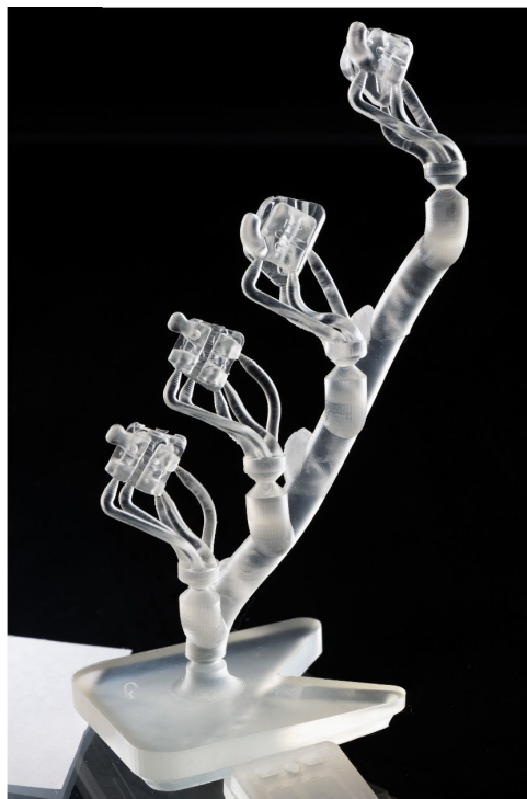
Figure 2. 3D Printed Customized Appliances. Customized indirect bonding system Monolithic – Braces on Demand (Braces on Demand Inc., Hicksville, NY). Brackets and indirect bonding trays are printed at the same time.
