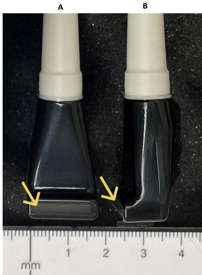
Figure 5. A) Illustration of the intra-oral ultrasound probe in a lateral view, and B) in a superior view. The arrows indicate where the sound waves are emitted from.
