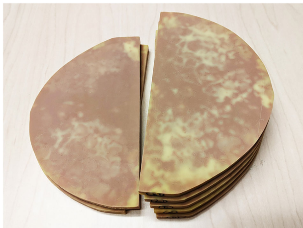
FIGURE 1 Modular breast phantom set with 1-cm-thick slabs of heterogeneous distribution of breast-tissue-equivalent material simulating a nominal 50% adipose/50% fibroglandular composition (custom-made by CIRS, Inc.).
