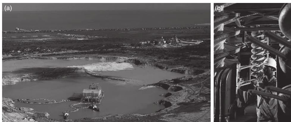
Figure 9.9 (a) The Moma titanium operation mines ilmenite, rutile, and zircon from beach sands along the northeast coast of Mozambique. The dredge shown here scrapes sand from the bottom of the water-filled pit and sends it through a pipeline to a concentrating plant. (b) Concentrating plant at the Moma operation showing spiral sluices down which the sand slurry flows. Heavy minerals move to the outside of the spiral and are captured. Waste sand is used to fill the mining pond, which advances into unmined sand (photographs courtesy of Kenmare Resources plc). See color plate section.
