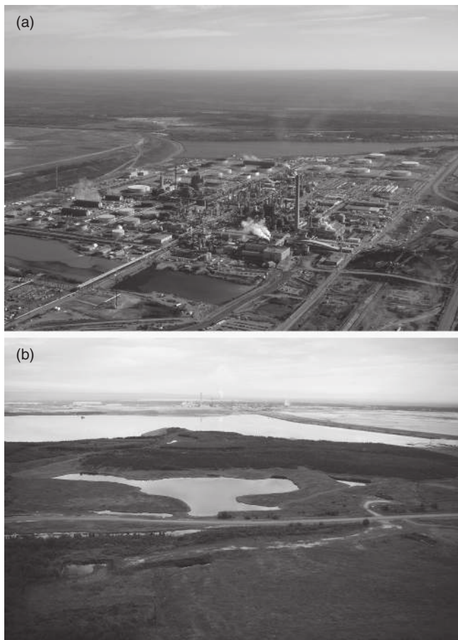
Figure 7.26 Tar sands. (a) Overview of processing plant with partly revegetated waste pile on left. (b) Reclaimed mined land with as yet unreclaimed waste dump on right. Processing plant is distant background (photos courtesy of Syncrude Canada). See color plate section.
