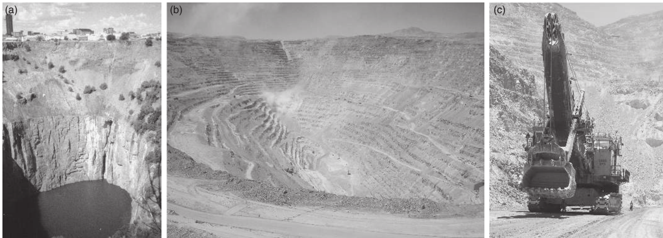
Figure 6.1 (a) The Kimberley mine in South Africa, began as small diggings that gradually grew to form the deep pit shown here, which continues to depth as the underground mine shown in Figure 11.18. The dark, high-rise building in the background is Harry Oppenheimer House, where diamonds from South Africa and Botswana are sorted and graded (photograph by the authors). (b) The Chuquicamata mine in northern Chile is one of several mines owned by US companies that were nationalized by the Chilean government in 1970 to form the state-owned corporation, Codelco. This mine, one of the largest in the world, measures 4.3 km long, 3 km wide and is almost 1 km deep. (c) This shovel is one of the tiny dots at the bottom of the Chuquicamata pit in the middle picture. The person standing below the bucket of the shovel, and another just beside it, show just how large this machine is (photographs by Antonio Arribas). See color plate section.
