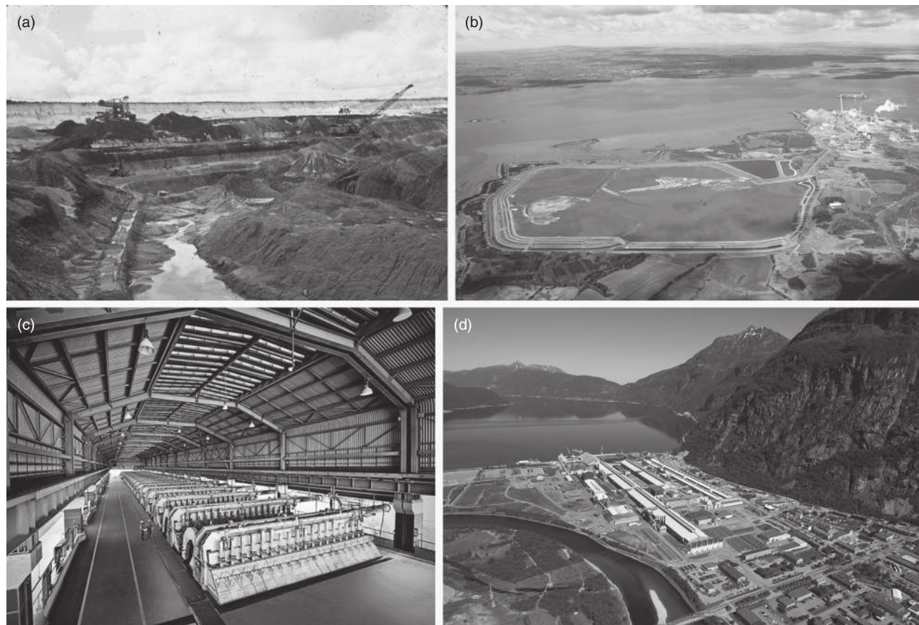
Figure 9.4 Aluminum production. (a) Strip mining of paleobauxite at MacKenzie, Guyana, which is buried beneath younger sediments. (b) Red mud waste from processing of bauxite, Aughinish, Erie (photograph courtesy of International Aluminum Institute). (c) Potroom where alumina is converted to aluminum, Dubai Smelter (photograph courtesy of International Aluminum Institute). (d) The largest aluminum refinery in Europe at Sunndalsora, Norway, uses hydroelectric power to process imported alumina (photograph courtesy of Oivind Leren/Hydro Sunndal). See color plate section.
