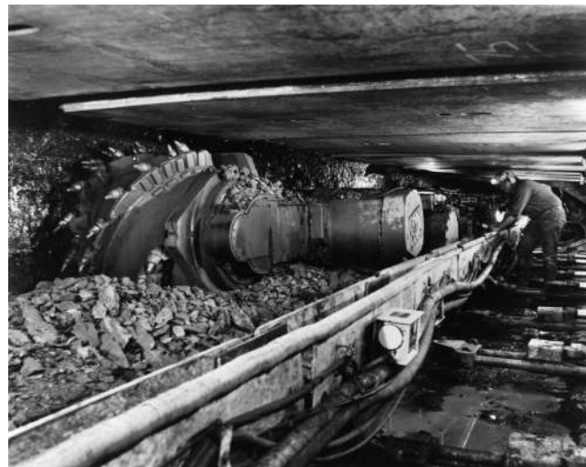
Figure 7.8 Underground longwall mine using a shearer loader. Note the cutting head at left and the hydraulic roof support canopy above the operator at right (courtesy of Bob Quinn, Eickhoff Corp.).
