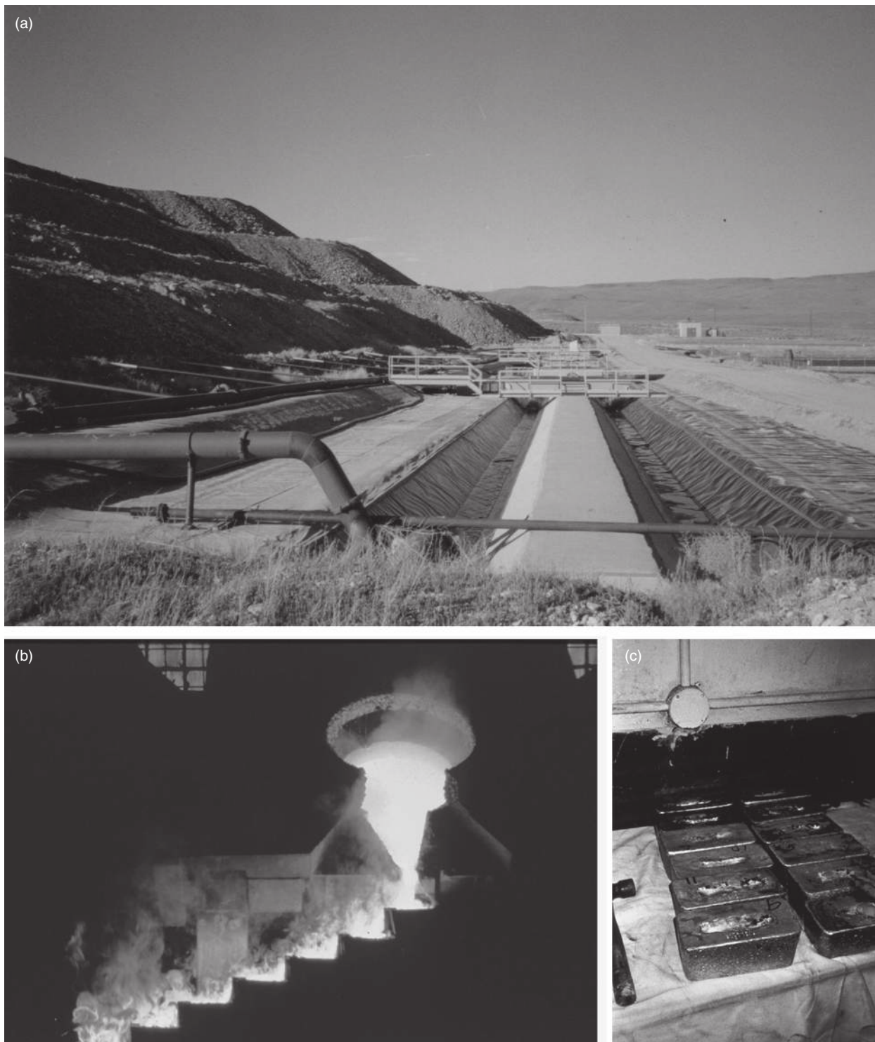
Figure 11.8 (a) Heap leach pads showing heaps of ore in left background. Cyanide solution is sprayed on the heaps, flows through the rock dissolving gold, and collects in the basins to the right foreground. Note thick plastic layer beneath the ponds and heaps to prevent recharge of solution into underlying groundwater. (b) Molten gold pouring from a furnace into molds. (c) Gold bars removed from molds. Each bar weighs about 27 kg and contains about 87% gold, 8% silver and small amounts of lead and zinc. The hand (lower right) provides scale (photos by the authors). See color plate section.
