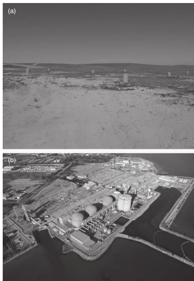
Figure 7.31 (a) Uranium mining by ISL. The barrels cover well heads that pump oxidizing water into the outer perimeter of the buried uranium deposit. The water flows through the deposit, leaching uranium, and then returns to the surface through wells in the center of the field. The entire field is surrounded by monitoring wells to detect and prevent any leakage of leach fluid beyond the deposit (photo by the authors). (b) The Pickering nuclear power plant on the north shore of Lake Ontario in Canada contains six operating and two inactive CANDU nuclear reactors with a total output capacity of 3,100 MW. The reactors are enclosed in the eight domed buildings, which are constructed of reinforced concrete. The large, light colored cylindrical building is a vacuum enclosure that is connected to the eight reactor enclosures. Any accidental release of radioactive steam from the reactors would be sucked into the vacuum enclosure rather than escaping into the atmosphere (photo courtesy of Ontario Power Generation). See color plate section.
