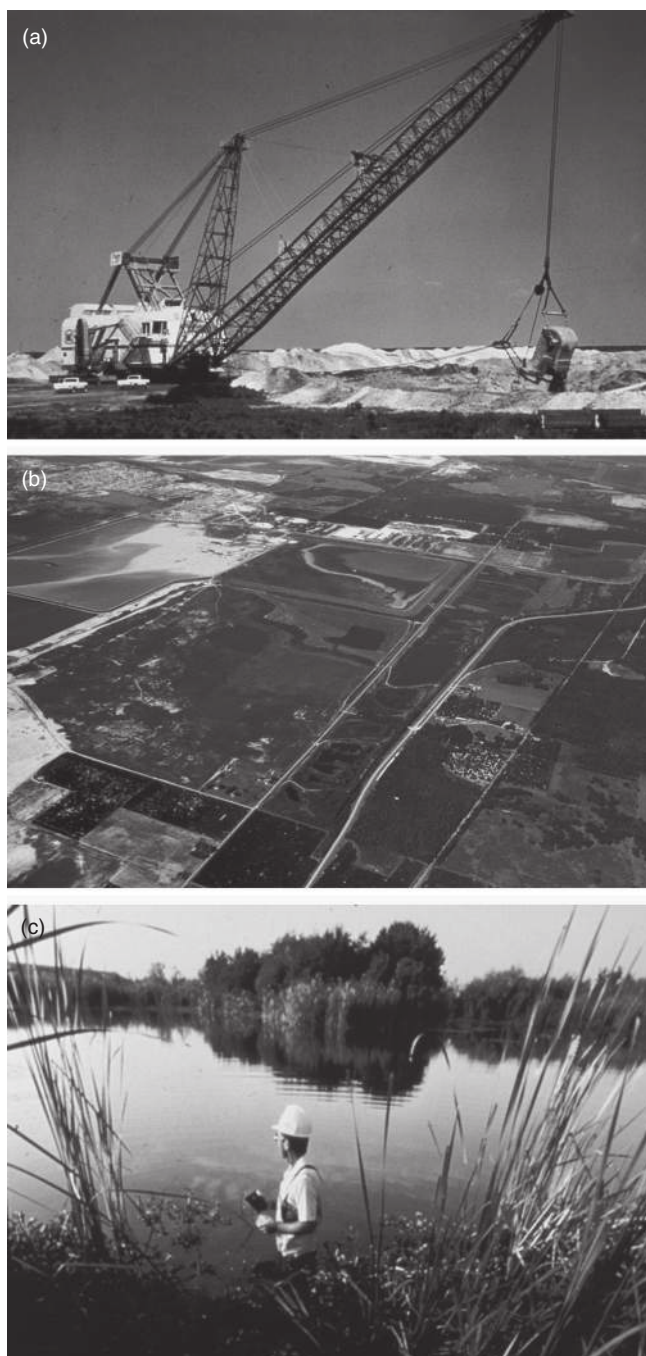
Figure 12.13 (a) Dragline moving overburden from phosphate mine in central Florida. (b) Overview of phosphate mine in central Florida showing active mining in left corner and two settling ponds where land is being reclaimed (lakes in center). Most other land has already been mined and reclaimed, usually as wetlands, the form in which it began. (c) Close-up view of reclaimed wetland on the site of a former phosphate mine in central Florida (photographs courtesy of Mosaic Corporation). See color plate section.
