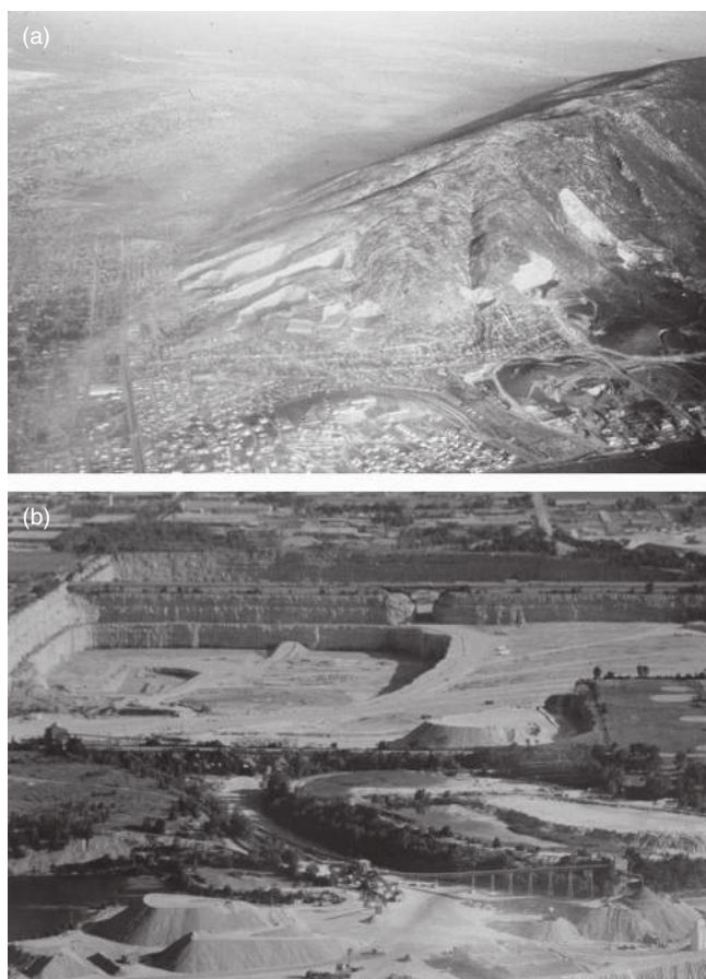
Figure 13.5 (a) Aggregate quarries on the outskirts of Monterrey, the third largest city in Mexico. Although the quarries were located perfectly from an economic standpoint, they created too much particulate pollution (note plumes of dust coming from the quarry at left) and most were closed during the late 1980s. (b) Aggregate quarry on the south side of metropolitan Chicago. This quarry is divided into two parts by a rib of rock left that supports Interstate 80, which can be seen in the background. A tunnel through the ridge, seen in the center, background, allows access to both parts of the mine (photos by the authors). See color plate section.
