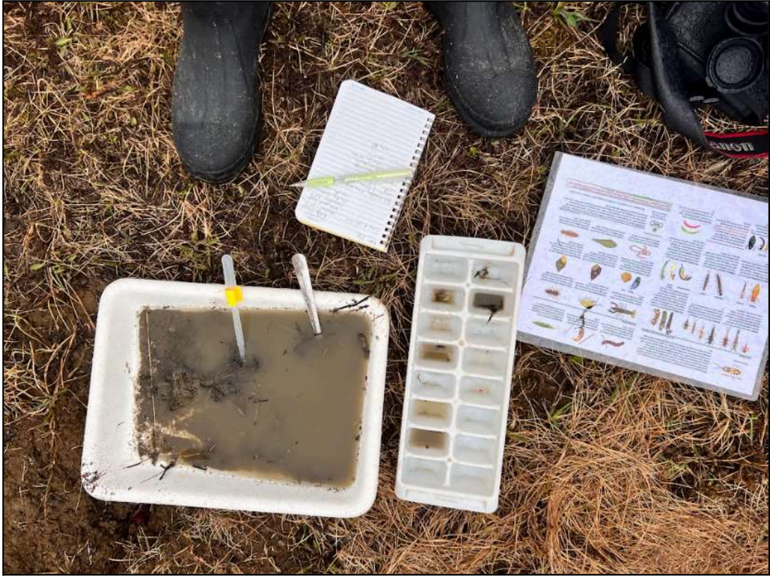
Figure 9. All materials used for benthic macroinvertebrate sampling (ice cube tray, paint tray, spoons, ID sheet). Not pictured: “D” Nets
