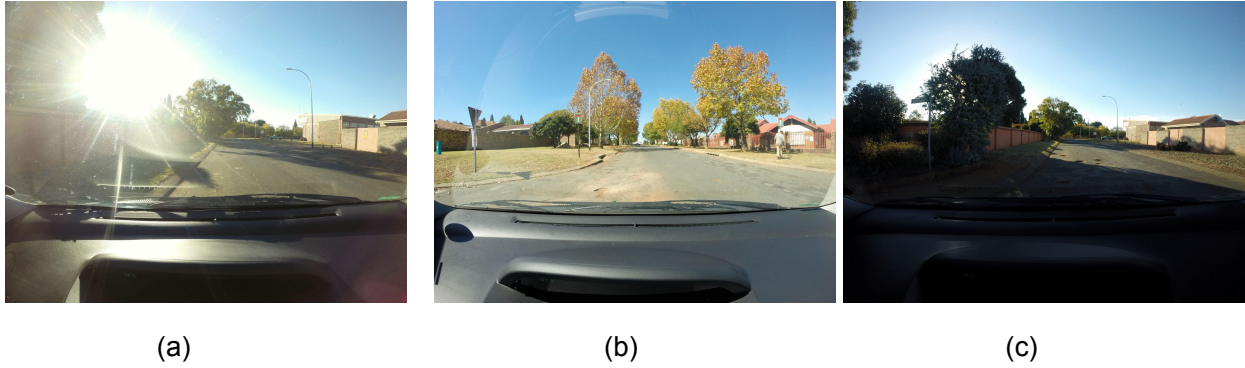
Figure 3.7: Examples of different images under different lighting conditions. (a) Image with sun rays towards the camera and low light covers the potholes, and (b) Clear light condition, and (c) Shadow covers potholes.
