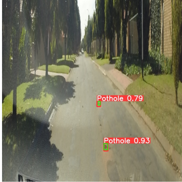
Figure 5.1: Plot of area overlap between the ground truth bounding boxes in green, and the predicted bounding boxes in red.
