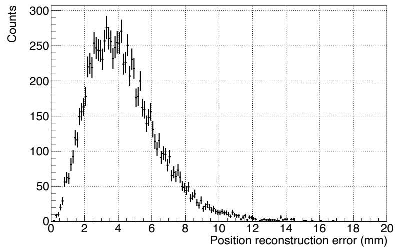
Figure 6.11: Distribution of position reconstruction errors using the CoM method for a point-like event comprising approximately 20000 initial photons near the center of the detector, with a mean of 4.35 mm and a standard deviation of 2.15 mm.
