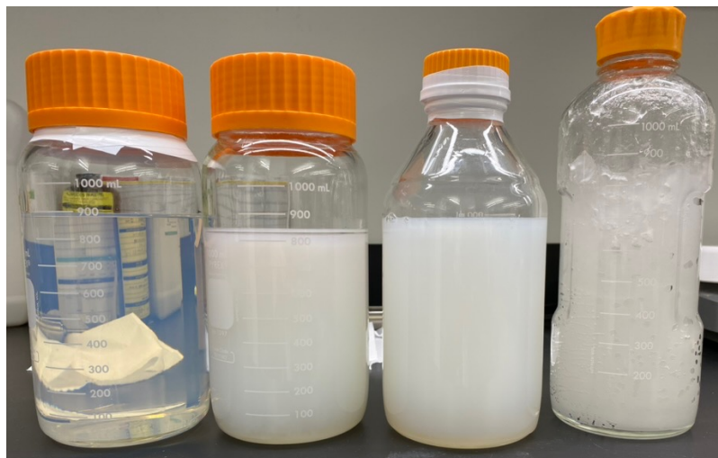
Figure 6.2: From left to right: oWbLS1, oWbLS2, oWbLS3, and NoWASH-20. oWbLS1 has the longest scattering length of the three oWbLS samples and appears relatively transparent, and oWbLS2 has the shortest scattering length. The waxy consistency of NoWASH-20 at room temperature ( \sim 18^\circ \text{C} ) can be observed.
