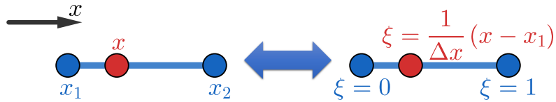
Figure 2.1: Mapping from physical space to reference space for a one-dimensional element.
