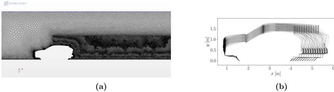
Figure 4.9: Pertaining the training dataset, (a) an example unstructured CFD mesh and (b) a composite image of all 124 vehicle shapes overlain on the same axes
