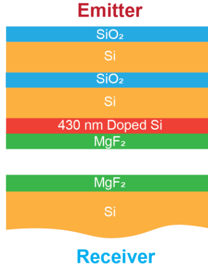
Figure 3-7. Schematic representation of the different layers considered in the theoretical calculations of near-field radiative heat transfer for the MgF 2 coated emitter and receiver devices.
