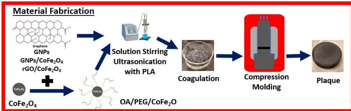
Figure 2-1 Process of design and optimization of PLA/GNPs/COE metamaterial absorbers
