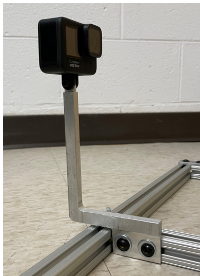
Figure 3.3: Sample attachment for capturing data in a vertical laser sheet
