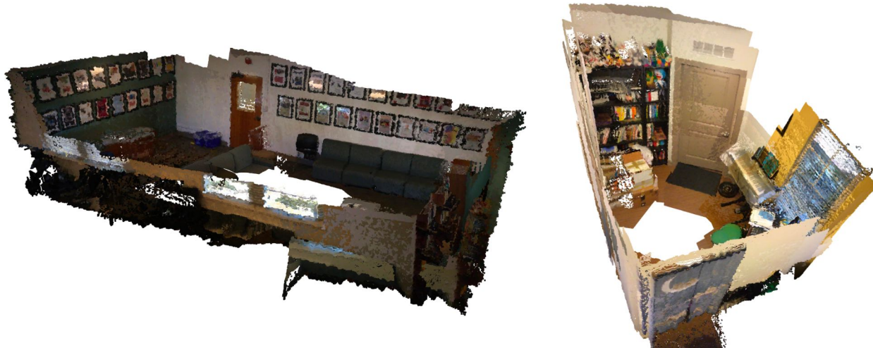
Figure 4.6: RGB-D Scene Reconstruction. SyncMatch can scale at inference time to longer videos to reconstruct longer sequences.
