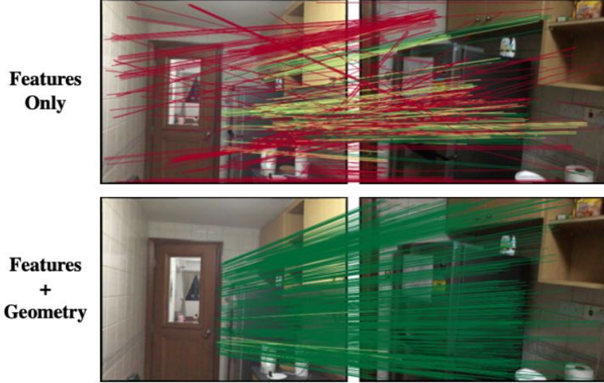
Figure 4.4: Geometry-aware sampling greatly improves our correspondence set. GART allows us to extract accurate correspondence even if the initial feature matches are very noisy.
