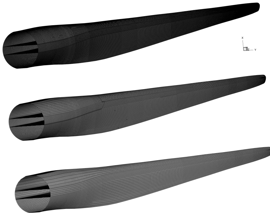
Figure 3.9: The structural mesh family, showing L0, L1, and L2 from top to bottom.
