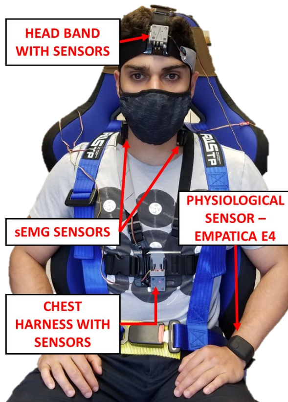
Fig 4-11 Demonstration of the instrumentation used to track passenger position and physiological response. Detailed view of the torso instrumentation and wrist based physiological sensor to track heart rate and perspiration of the occupant
