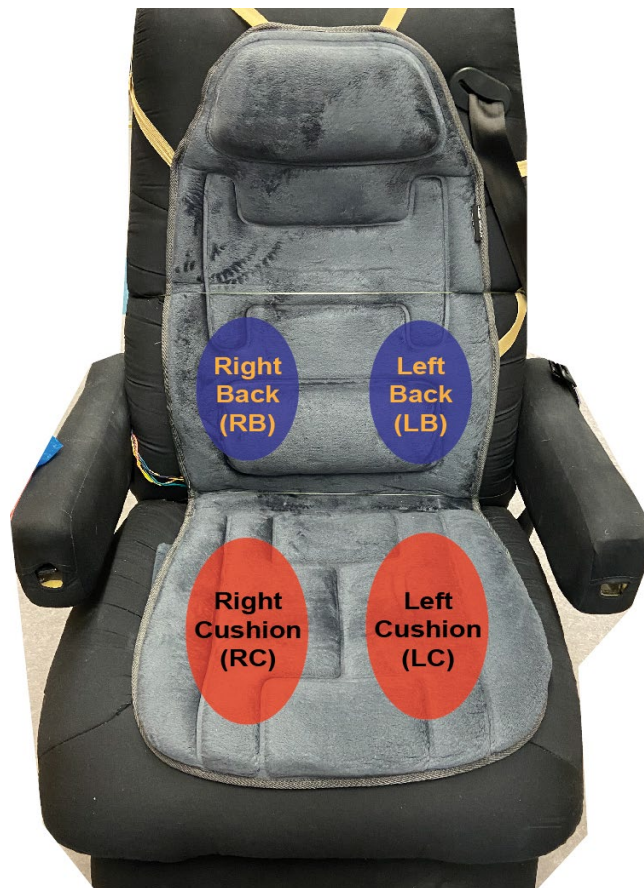
Fig 5-1 Haptic Stimuli System using commercially available Seat Cover
