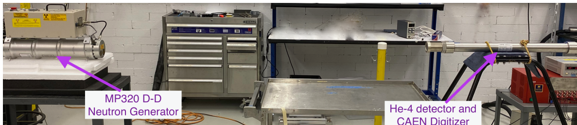
Figure 2.3: An example experimental setup, showing the ^4\text{He} detector and its associated electronics (right) and the MP320 D-D neutron generator (left). The generator is elevated from the laboratory floor using a steel lab cart and several layers of low-density polyurethane foam and polystyrene foam such that the center of the generator target is at the same elevation as the center of the detector.
