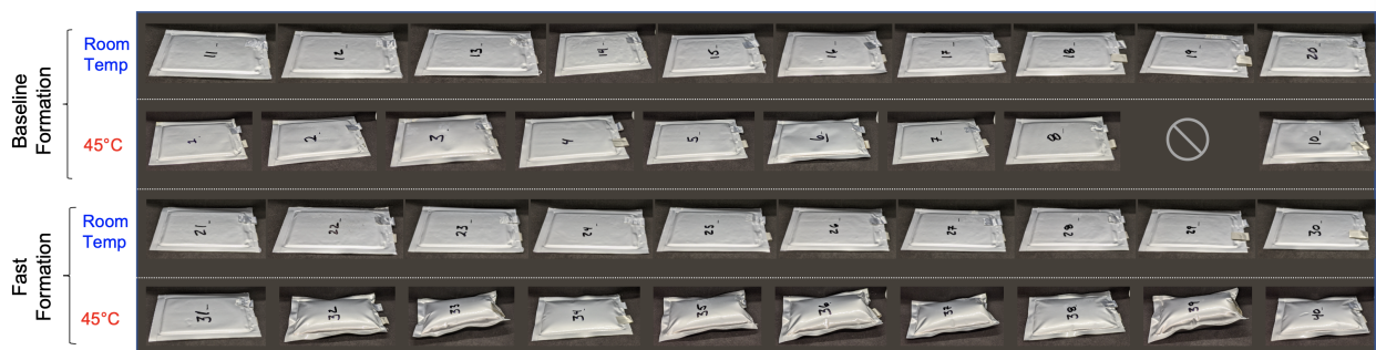
Figure B.26: Images of pouch cells taken after aging. Cell #9 has been excluded from the study due to tab weld issues.
