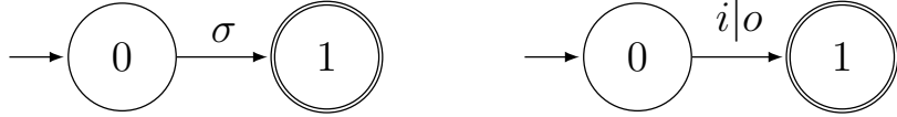
Figure 2.1: An example automaton G (left) and transducer T (right). Marked states are denoted by double outlines. So the marked language of G is \mathcal{L}_m(G) = \{\sigma\} . In the transducer, the notation i|o represents an input i resulting in output o . So the marked relation of T is \mathcal{R}(T) = \{(i, o)\} .
