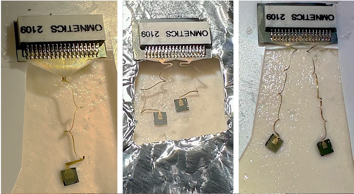
Figure 3.38: Implantation of high-density electrode arrays into tofu, showing the shanks robustness and the flexibility of the meandered cables.
