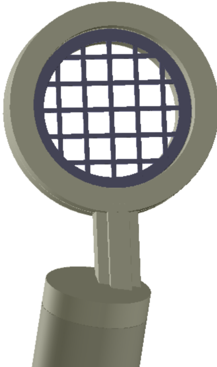
Figure 4.9: VisRad illustration of the configuration used for experimental calibration. A copper mesh target was used to determine the resolution of the radiography setup. The mesh strips are 0.08 mm wide and 0.02 mm thick.
