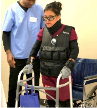
Figure 1.2: Example of simulated impairment. An age-simulation suit is shown, along with the simulated need for an ambulation aid (i.e., the walker) and a mobility aid (i.e., the manual wheelchair).
