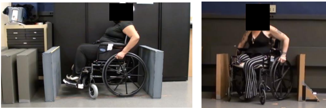
Figure 4.1: A MWU participant maneuvering into the parallel parking space. A cardboard panel is seen on either side of the space. (Left) First version, utilizing pre-existing panels; (Right) Second version, utilizing new, narrower panels.
