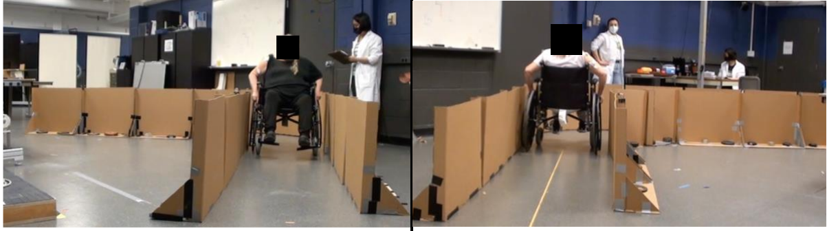
Figure 5.2: Illustration of the path-following task. One experimenter observes critical event counts while the other monitors sEMG signals to ensure safe levels of muscular exertion. The image on the left shows no intervention, and the image on the right depicts the “Mid-line marker” bottom-up intervention.
