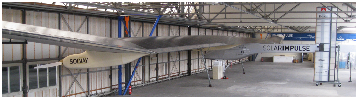
Figure 1.3: Lightweight, but not very flexible Solar Impulse 1 [3] (Photo by Matth1). The large volume and light weight of the structure required additional considerations to accurately capture the apparent mass effect.
