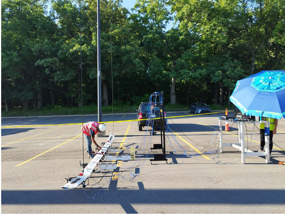
Figure 6.38: Side view of the X-HALE and the ground station during the free-free GVT. The accelerometer wires introduced additional stiffness to the system.
