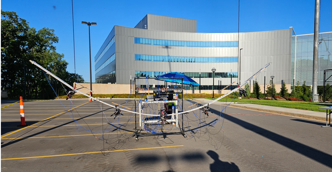
Figure 6.34: The X-HALE suspended in the outboard configuration during the free-free GVT, connected to the bungee cords dropped from the crane.
