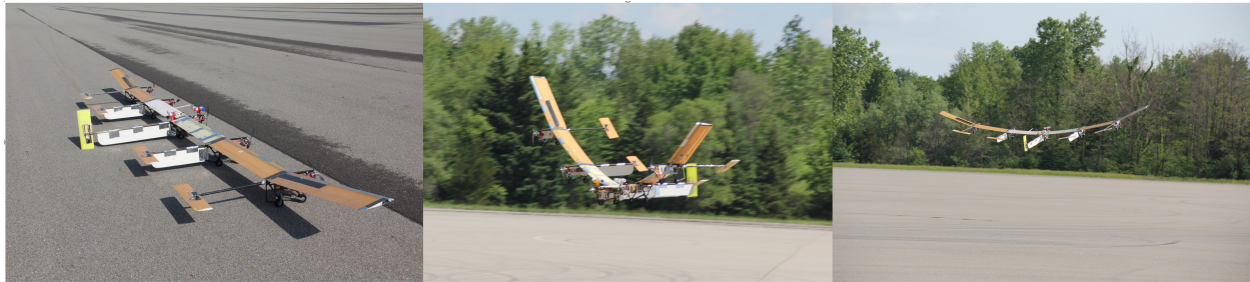
Figure 6.1: X-HALE airframe on the ground and in flight.
