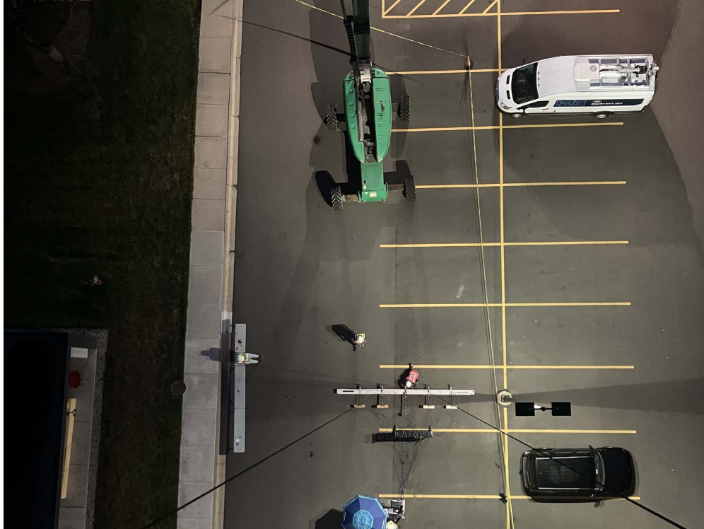
Figure 6.36: The X-HALE during the free-free GVT, as viewed from the crane.
