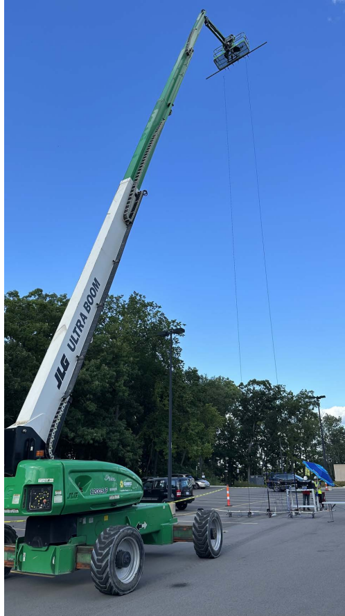
Figure 6.33: The crane with the X-HALE suspended from it during the free-free GVT.
