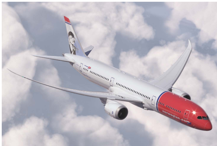
Figure 1.4: Boeing's 787 2 wing flexing during flight (Photo by Norwegian Air Shuttle).
