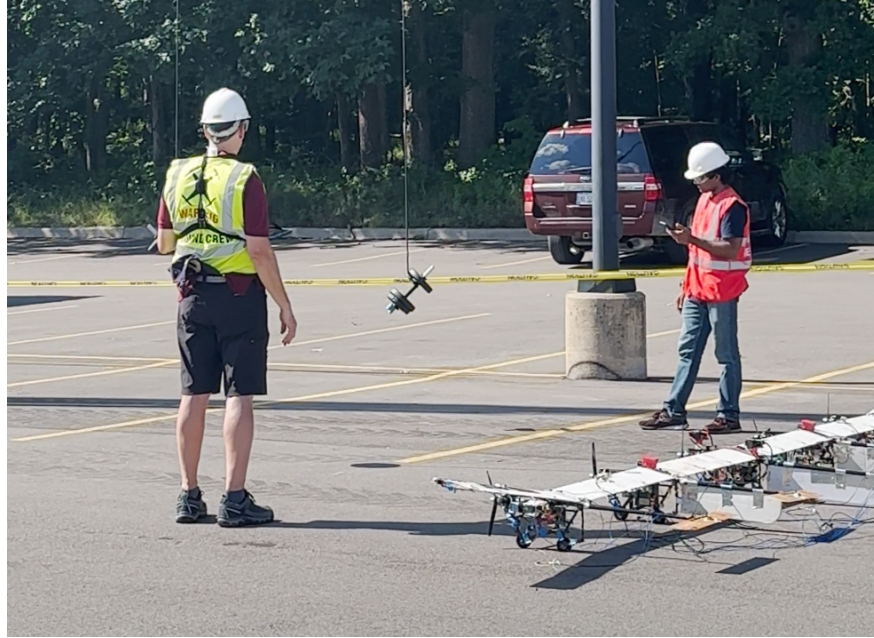
Figure 6.37: The calibrated mass (dumbbell suspended from bungee cord, middle of the image) used to measure the bungee plunge frequency.
