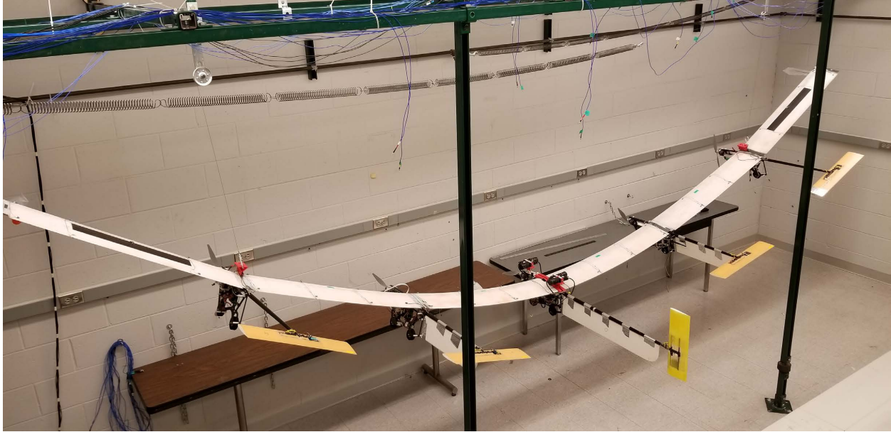
Figure 6.3: X-HALE suspension setup.
