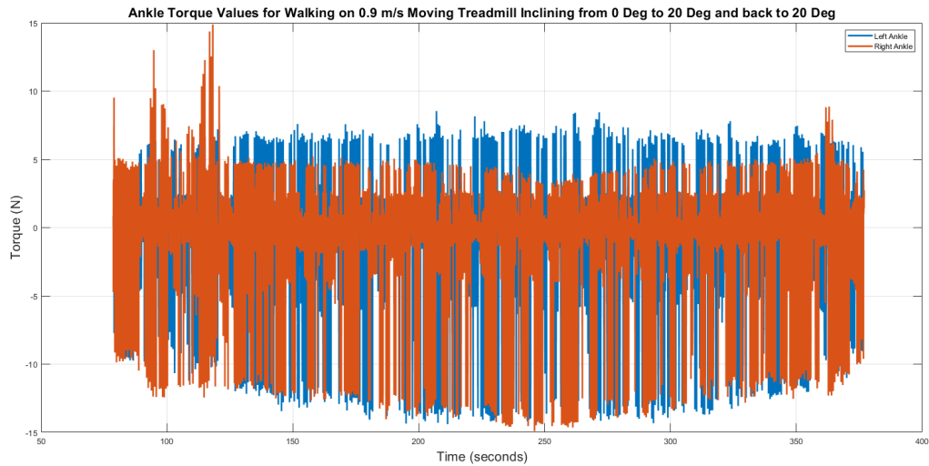
Figure 5.3: Plot of left and right ankle torque values for hardware experiment on the Cassie bipedal robot walking on an inclined moving treadmill moving at a constant speed of 0.9 m/s. The treadmill is gradually inclined from 0 degrees to its maximum incline of 20 degrees and back to 0 degrees.
