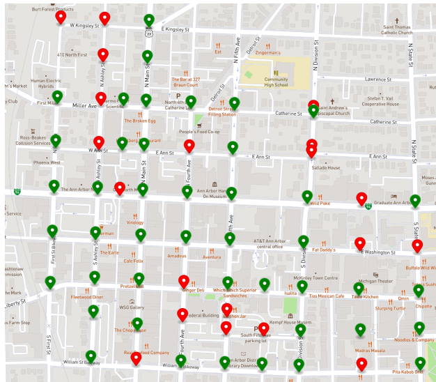
Figure A.3: Spatial distribution of intersections under the stochastic model solution with delay improved or unchanged compared to the baseline in the traffic network during morning peak hours, marked by green color in the figure.
