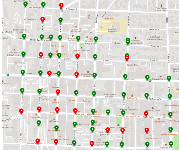
Figure A.5: Spatial distribution of intersections under the stochastic model solution with delay improved or unchanged compared to the baseline in the traffic network during off-peak hours, marked by green color in the figure.
