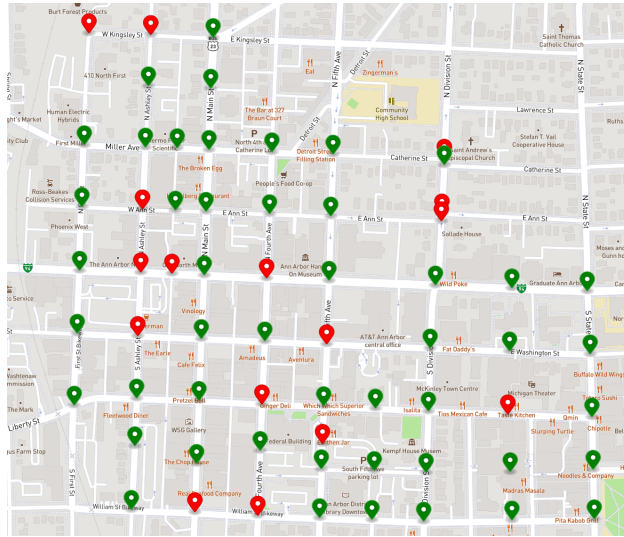
Figure A.9: Spatial distribution of intersections under the stochastic model solution with delay improved or unchanged compared to the baseline in the traffic network during afternoon peak hours, marked by green color in the figure.
