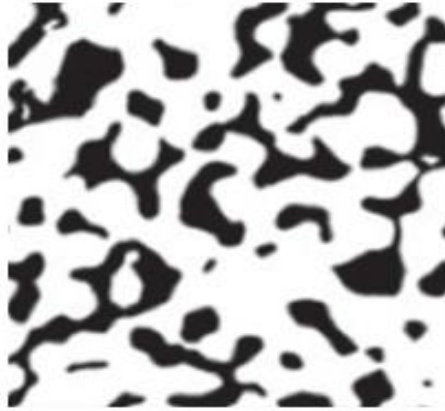
Figure 1-7 The microstructure of space(black) between ice(white) from microscopic imaging[83,84].
