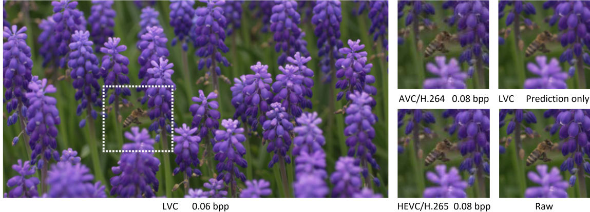
Figure 3.1: Reconstructed frame with the conventional codecs (H.264, H.265) and LVC approach. Information and details are well preserved in the frame generated from a purely prediction-based latent representation (top right).
