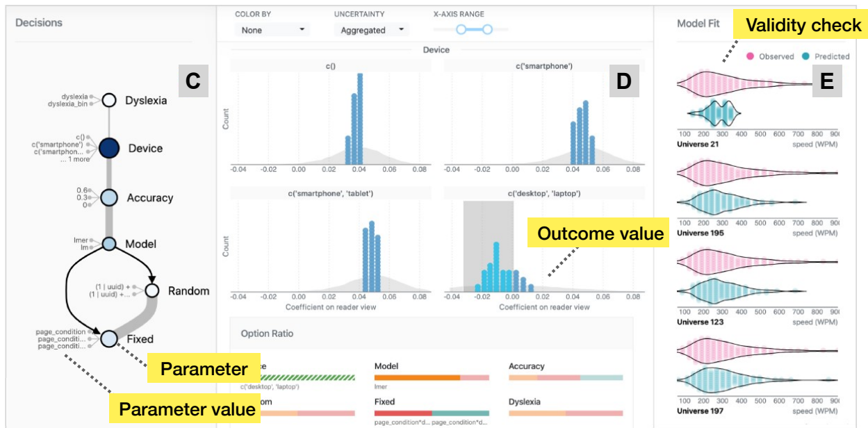
Figure 3.15: Screenshot of the Boba system [58]. Panel C shows the design space of parameters and their relationships; parameters that are source of sensitivity are in a darker color. Panel D is a trellis of dotplots of outcome values, subsetted by parameter values. Panel D shows predictive distributions from each universe compared to the observed data.
