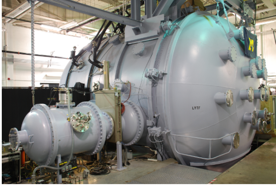
Figure 3.2: Large Vacuum Test Facility at the University of Michigan
