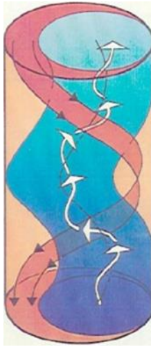
Figure 3-28 EPRI representation of double helix like flow in the branch line where both upward and downward flow are entrained in the same swirl.
