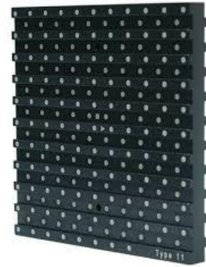
Figure 2-11 Double-sided 3D calibration target.
