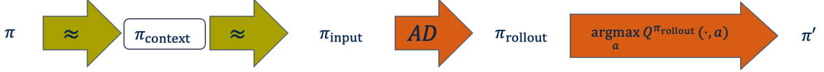
Figure 20: Diagram of the policy improvement cycle. The behavior policy \pi generates new actions and the environment generates new transitions which are appended to the front of the context window. By retaining only the most recent transitions in the context window, we ensure that the policy represented in the context approximates the behavior policy. Next, we rely on the policy improvement operator learned by the transformer to infer the distribution of actions in the context and yield an improved action for our rollout policy. Therefore the rollout policy approximates the prompt policy. Finally, by choosing actions greedily with respect to our value estimates, we implement a new behavior policy \pi' that improves the rollout policy.
