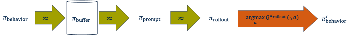
Figure 7: Diagram of the policy improvement cycle. The replay buffer is fed by a behavior policy. Next we sample the trajectories used in the policy prompt from recent episodes in the buffer. By sampling recent episodes only, we try to keep the prompt policy close to the behavior policy. Next, we rely on the language model to infer the distribution of actions in the prompt and yield a similarly distributed action for our rollout policy. Therefore the rollout policy approximates the prompt policy. Finally, by choosing actions greedily with respect to our value estimates, we implement a new behavior policy that improves the rollout policy.
