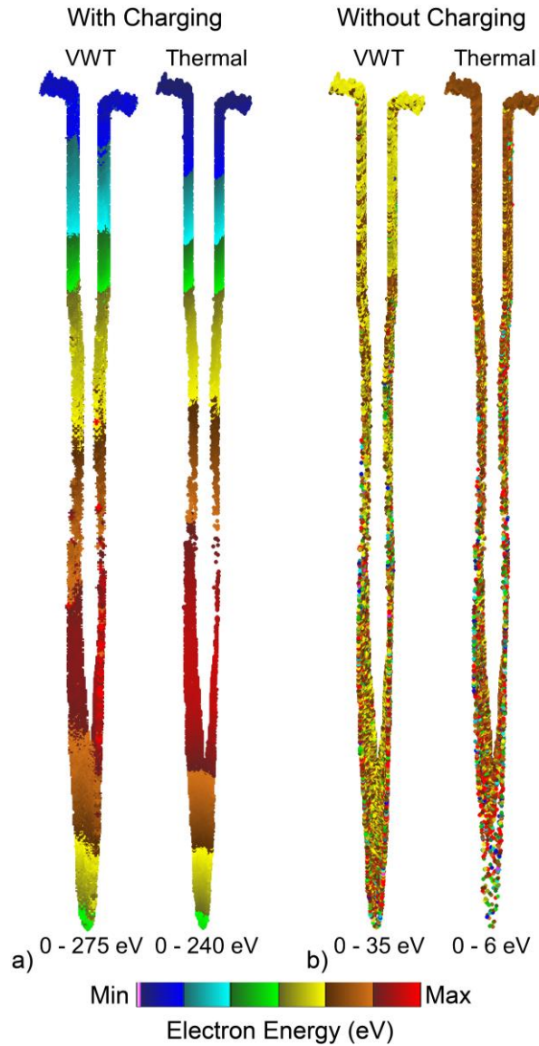
Figure 4.8: Spatial distribution of average electron energies incident on the surface of the feature. The feature properties are for P_{VWT} = 1000 \text{ W} and \varphi = 0^\circ after 15 minutes of etching. Results are shown for initial EEADs produced with VWT and for thermal electron having a temperature of 3 eV. a) When including acceleration in electric fields produced by feature charging. b) Without acceleration due to feature charging. The view is looking obliquely into the 3-dimensional feature having reflective boundary conditions front-and-back.
