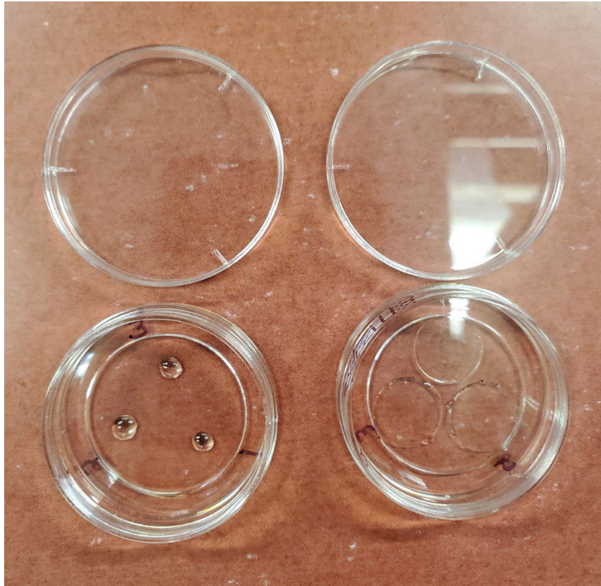
Figure 2.4: PDMS-coverslip Mounting Arrangement Diagram. Mounting configuration of PDMS-coated coverslips onto 35-mm glass bottom dishes. Three dots of mounting solution can be applied to each 35-mm glass bottom dish (bottom left) and PDMS-coated coverslips mounted face down onto the 35-mm dish such that the cells are mounted against the glass bottom dish (bottom right), allowing for imaging of the cells on an inverted microscope without negative effects associated with imaging through the PDMS layer.
