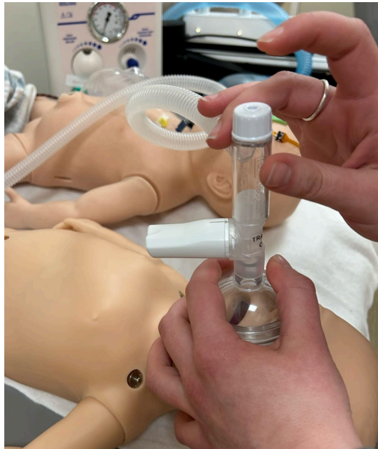
Figure 42: Air leakage testing done on just the manikin itself.
