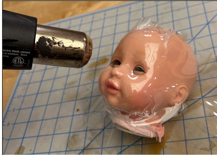
Figure 27: Thermoforming process of a TPU sheet to the doll's head with a heat gun.
