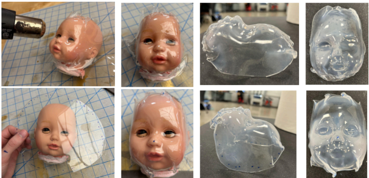
Figure 28: The first row of images shows the thermoforming process and result of our first trial. The second row of images shows our second trial.
