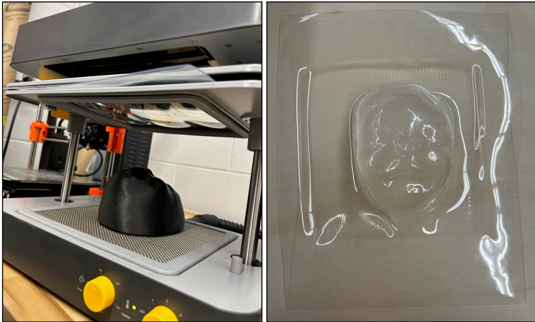
Figure 30: 3D model of manikin being vacuum formed in the MBSE Leadership Lab (Left). Results immediately after vacuum forming (Right).
