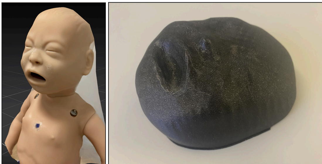
Figure 29: STL model of SimNewB manikin (Left). 3D print of scanned face (Right).
