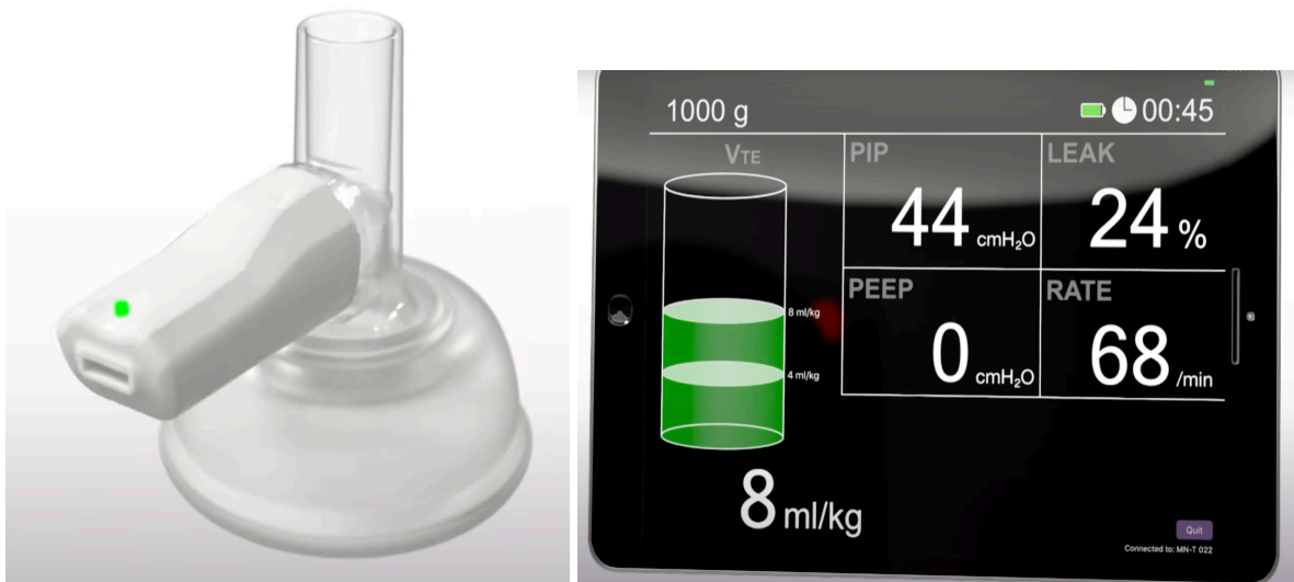
Figure 36: Sensor module that attaches to the ventilation mask (left). Display screen with continuous feedback and air leakage percentage shown in top right (right).
