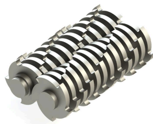
Figure 24. Above shows the staggered shredding blade orientation on a dual-shaft shredding machine. This orientation ensures that no more than one tooth is in contact with the firearm at the same time, which allows the shredder to maintain the applied shear stress on the firearm [42].
