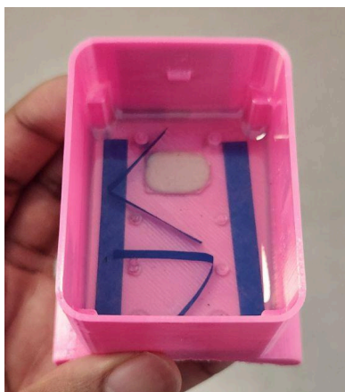
Figure 27: The potted blue cobalt chloride strips after waterproof testing. Note that the color of each strip remained blue, indicating no moisture within the potted packaging and thus verifying that this packaging method is waterproof.
