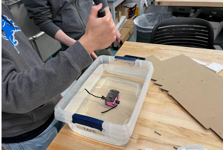
Figure 28: The fully encased C-HAT submerged in water to confirm electronic function underwater.
