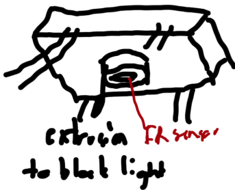
Figure C14: Sketch of C-HAT with opaque extrusion around the IR sensor to block ambient light.
