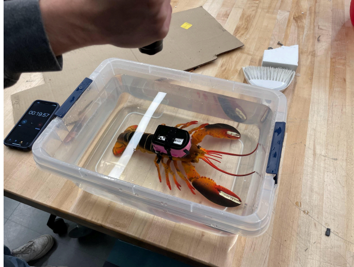
Figure 30: The fully encased C-HAT mounted on the model lobster and submerged in water to confirm the interface's ability to filter out IR light underwater.
