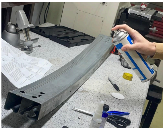
Figure E.1: Application of degreaser. The degreaser would then be wiped using a cotton pad.
