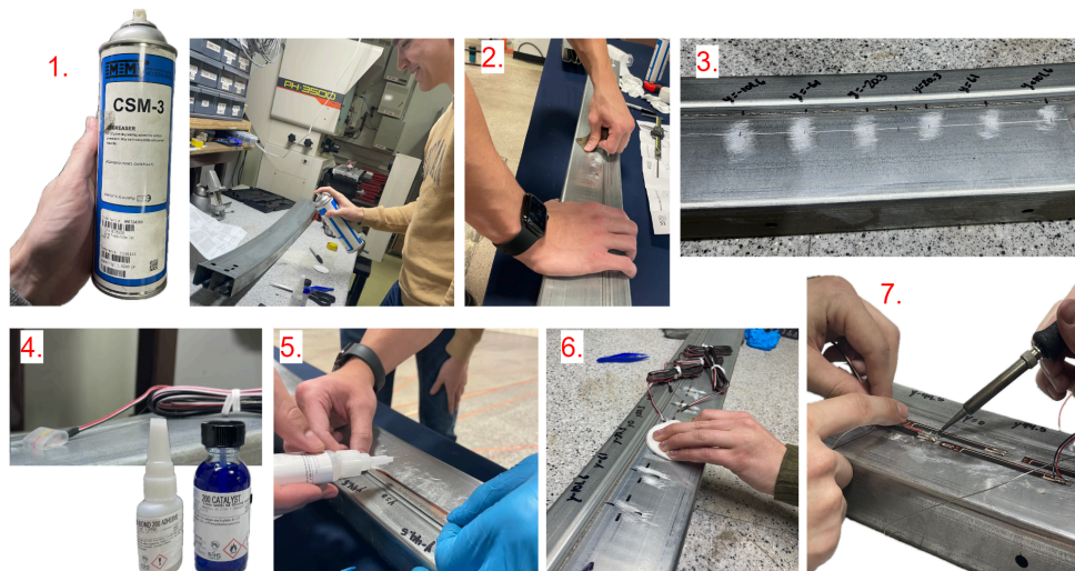
Figure 13.1: Installation process of strain gauges and flex sensors followed on Tuesday, March 12 th , 2024.
