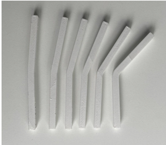
Figure 11.6: A sample set of the implements used to bend the Flex Sensors at specific angles. The angles shown here at 5, 10, 15, 20, 30, and 45 degrees, with a 1 cm radius of curvature.
