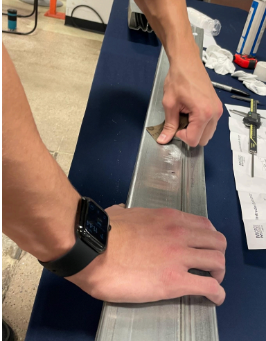
Figure E.3: Roughen the strain gauge placement locations with sandpaper
