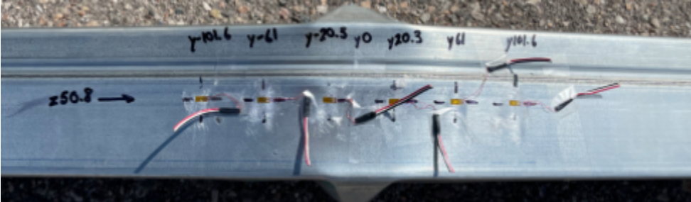
Figure 12.1: Strain Gauge Build Design Post Testing. This picture showcases the 6 strain gauges each adhered to their specified locations, and proves that the sensor build design stays intact throughout testing.
