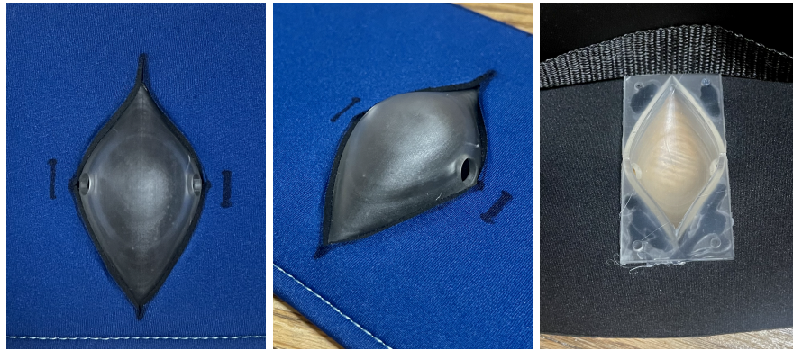
Figure 46. Initial packaging prototype (resin printed) inserted into neoprene collar using hot glue in place of any adhesives used and before sewn in.
