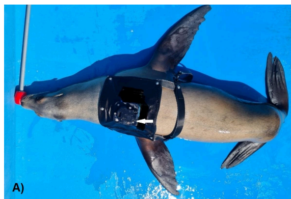
Figure 24. Sea lion wearing current harness design, D-tag attached at top with hydrophones facing backside *Videos adapted from given footage given by Dr. Kastelein **Images adapted from [2]
