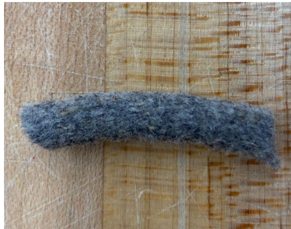
Figure 22: The wick used by Heller Industries to lubricate the chain external to the vacuum chamber
