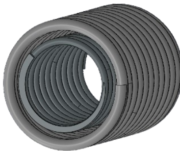
Figure A2. CAD image used to show the current two spring design.
