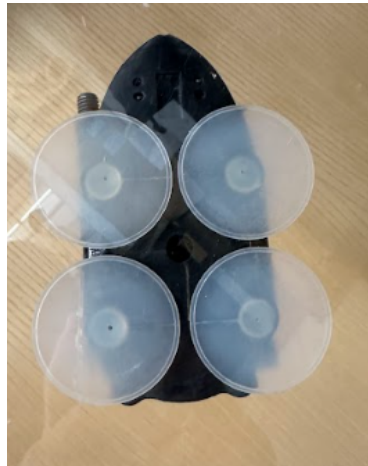
Figure 39: A picture of the suction quality for a successful drop. All four suction cups were fully depressed for this particular trial.
