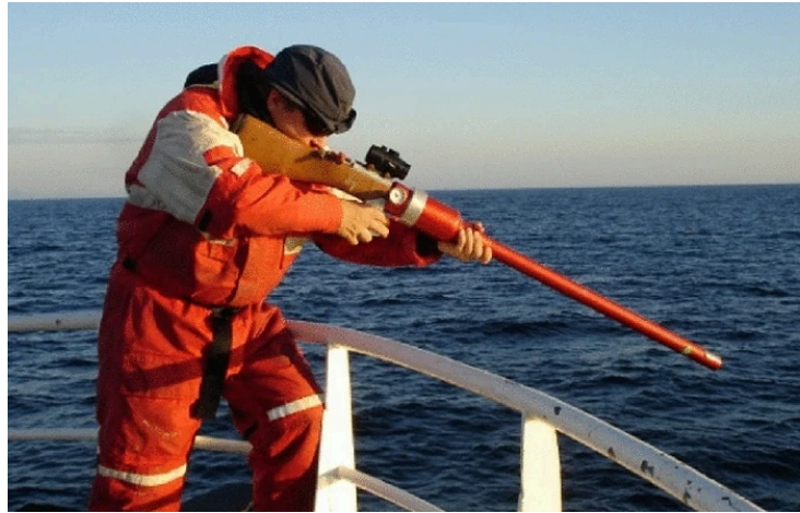
Figure 2: Researcher deploying a biologging device with a pneumatic gun from the deck of a vessel to tag an animal without physically contacting them [4].
