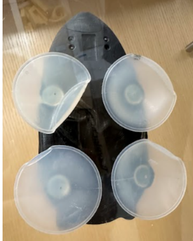
Figure 40: A picture of a trial that was considered successful but not ideal. The suction cups are folded over themselves which indicate that the DTAG might have been tilted upon impact with the acrylic.
