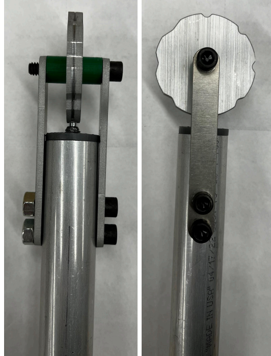
Figure 16. Completed Leg Joint subassembly with Wheel Joint V2
